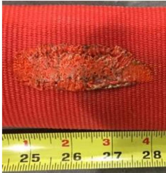
**Figure 9: TPU Hose Failure Example**
