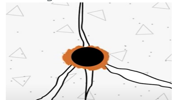
Figure 4. Rusting of steel-reinforced concrete 9
