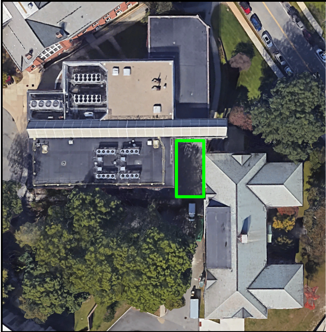
Figure 16. Potential green roof site between Fuller Laboratories and Kaven Hall as of May 2023
