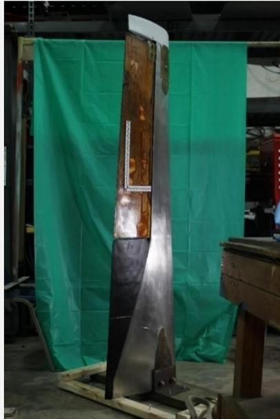
Figure 18: 45-degree view of the rotprop blade used as a reference to generate the CAD model.
