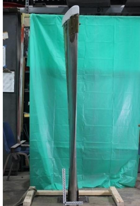
Figure 17: Perpendicular view of the leading edge of the rotprop blade used to generate the CAD model.
