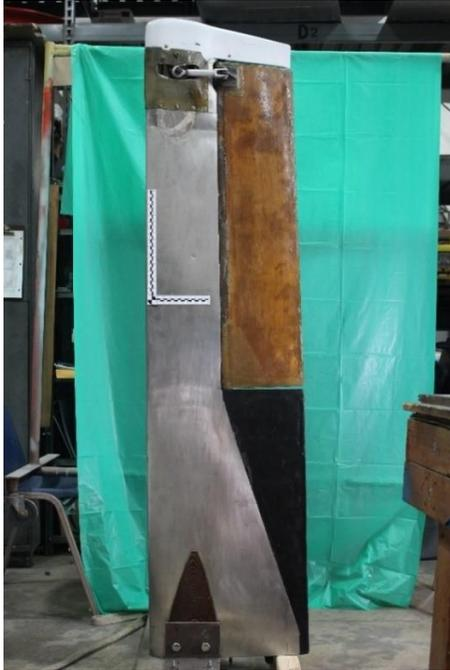
Figure 16: Perpendicular view of the underside of the rotprop blade used to generate the CAD model.
