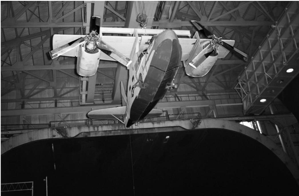
Figure 2: 3/4 front view of the K-16B in 40-by-80-foot wind tunnel at the NASA Ames Research Center [22].
