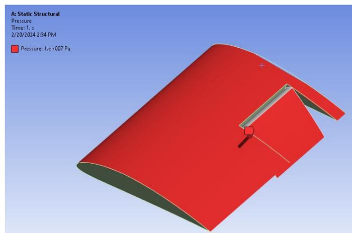
Figure 84: Uniform pressure load applied to sample model in practice static analysis.
