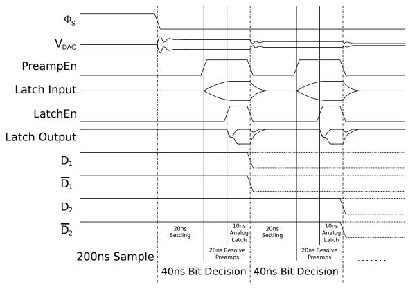
Figure 6.13: Timing Diagram of Control Signals
