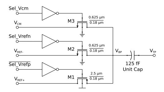
Figure 6.7: Switching Circuit for 125 fF Capacitors
