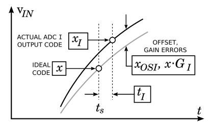
Figure 3.1: Effects of time interleaved channel mismatch on an input signal
