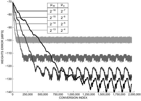
Figure 6.16: Split-SAR Algorithm Convergence with Different Waveforms
