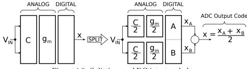
Figure 4.3: Splitting an ADC into two halves
