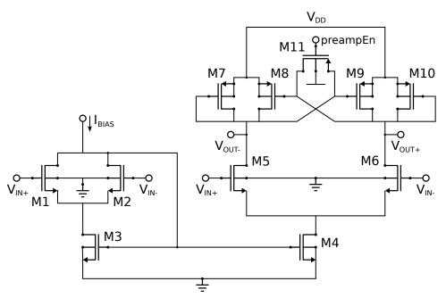
Figure 6.9: Preamplifier Single Stage Schematic
