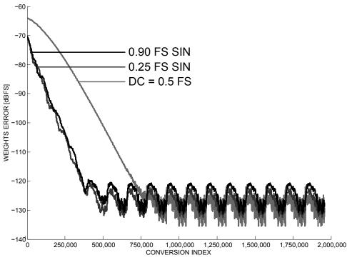
Figure 6.17: Split-SAR Algorithm Convergence with Different LMS Parameters
