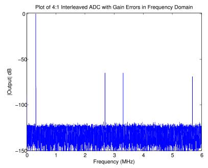
Figure 3.5: 4:1 Time Interleaved Output Spectrum with Gain Errors
