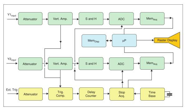
Figure 1.2: Block Diagram of a Digital Sampling Oscilloscope
