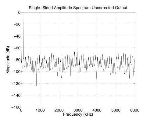
Figure 5.9: FFT of Uncorrected Sine Wave  $f_{in} = 140.625 kHz$
