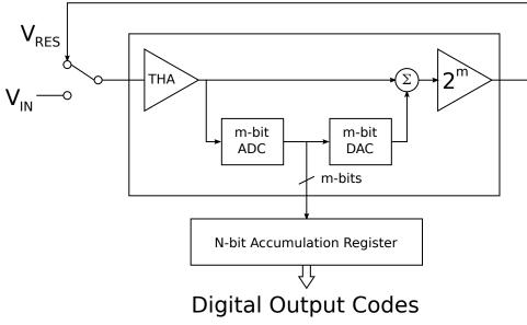
Figure 2.8: Block Diagram of a Cyclic ADC
