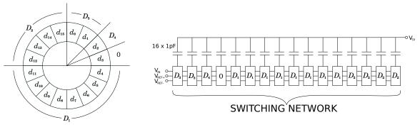
Figure 6.3: Split-SAR Bank Capacitor Selection
