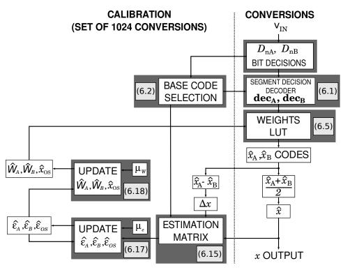
Figure 6.4: Split-SAR Error Estimation Algorithm and Correction
