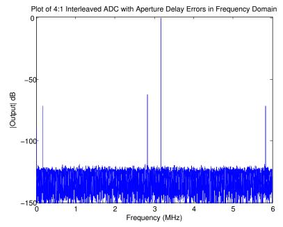
Figure 3.7: 4:1 Time Interleaved Output Spectrum with Aperture Delay Errors
