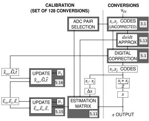
Figure 5.3: Error Estimation Algorithm and Correction
