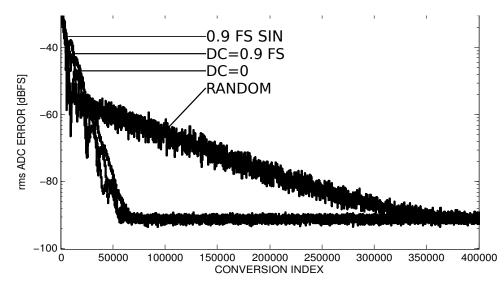
Figure 5.7: Calibration Convergence for Sinusoidal, DC, and Random Input Signals
