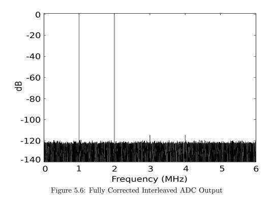
maximum bandwidth mismatch in this 16-bit system is  $\pm 1\%$ .
