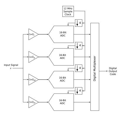
Figure 3.4: Block Diagram of 4:1 Time Interleaved Converter with Gain Error Introduced
