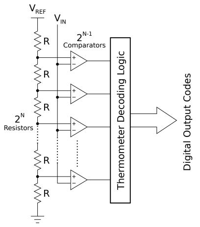
Figure 2.7: Block Diagram of a Flash ADC
