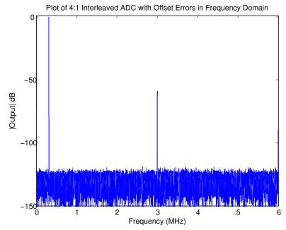
Figure 3.3: 4:1 Time Interleaved Output Spectrum with Offset Errors
