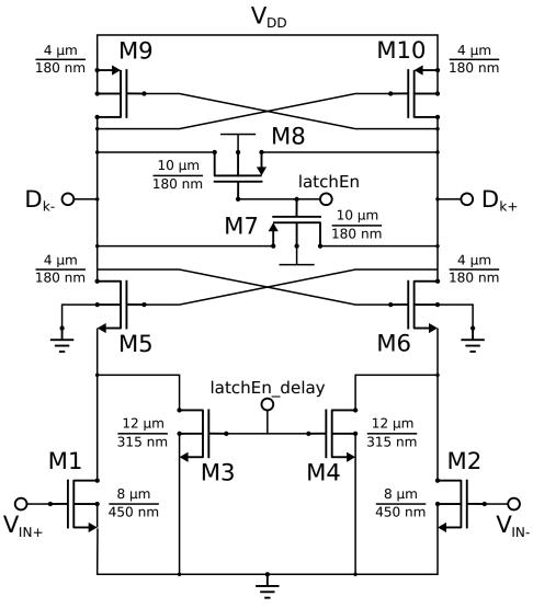
Figure 6.10: Preamplifier Regenerative Latch
