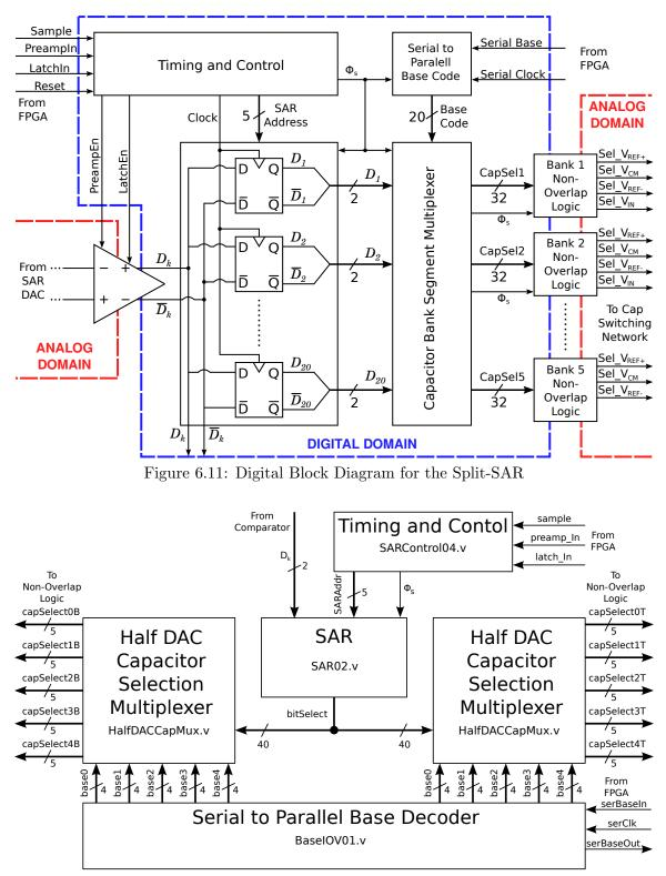
Figure 6.12: Digital Circuit Hierarchy Block Diagram
