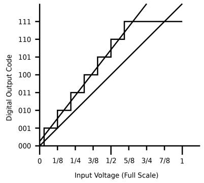
Figure 2.3: ADC Transfer Function with Offset and Gain Error.
