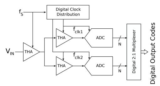
Figure 1.3: Block Diagram of a 2:1 Time-Interleaved ADC
