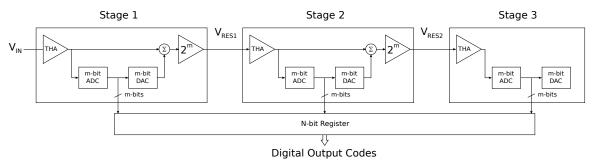
Figure 2.9: Block Diagram of a Pipelined ADC
