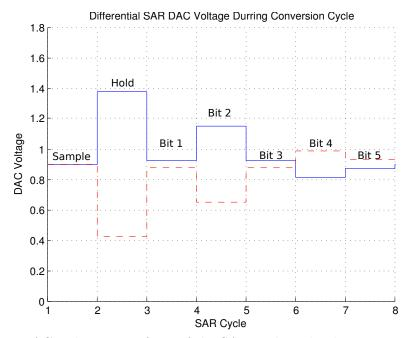
Figure 3.12: DAC Voltage Waveform of the SAR with Redundant Bit and Recovery
