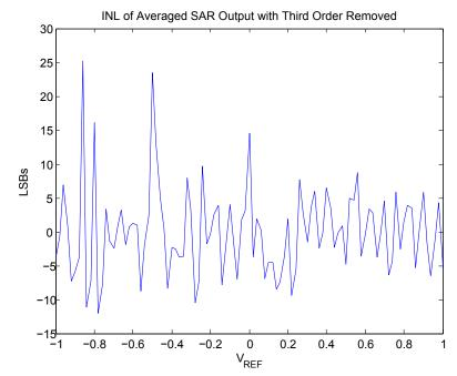
Figure 6.21: 100 Point INL of Calibrated Split-SAR with Third Order Effect Removed
