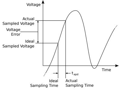
Figure 2.6: The Effects of Aperture Delay on the Sampled Voltage
