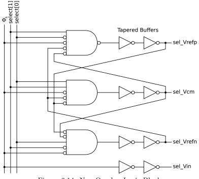
Figure 6.14: Non-Overlap Logic Block
