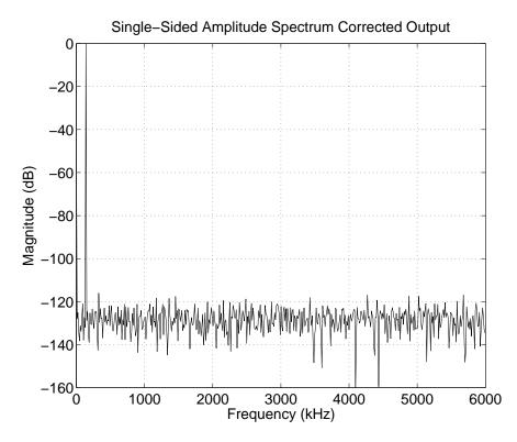
Figure 5.10: FFT of Corrected Sine Wave  $f_{in} = 140.625 kHz$
