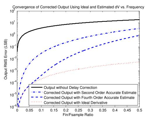
Figure 5.2: Comparison of Derivative Estimates used for Error Correction
