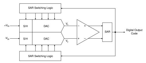
Figure 3.9: Block Diagram of a Differential SAR
