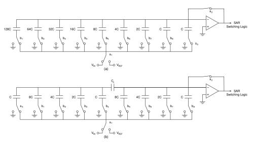
Figure 4.1: (a) An 8-bit SAR with straight binary weighted DAC (b) An 8-bit SAR with a Coupling Capacitor DAC
