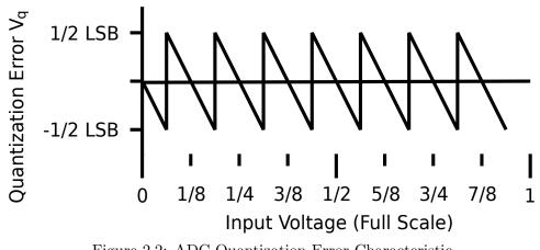
Figure 2.2: ADC Quantization Error Characteristic
