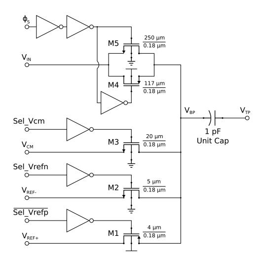
Figure 6.8: Switching Circuit for 1 pF Capacitors
