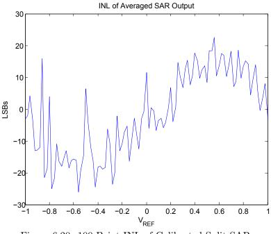
Figure 6.20: 100 Point INL of Calibrated Split-SAR
