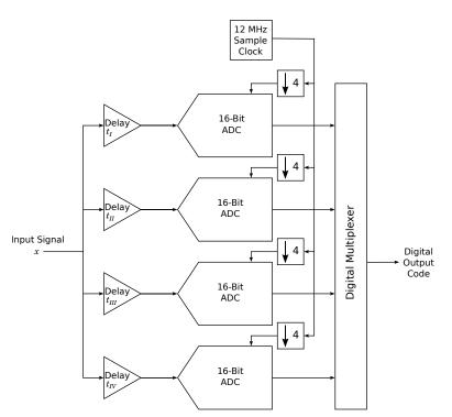
Figure 3.6: Block Diagram of 4:1 Time Interleaved Converter with Aperture Delay Error Introduced
