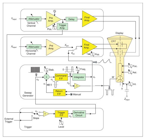
Figure 1.1: Block Diagram of an Analog Oscilloscope
