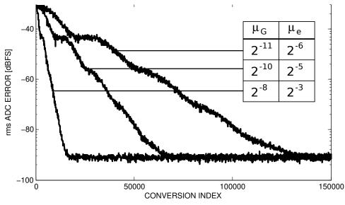
Figure 5.8: Calibration Convergence for Different LMS Parameters
