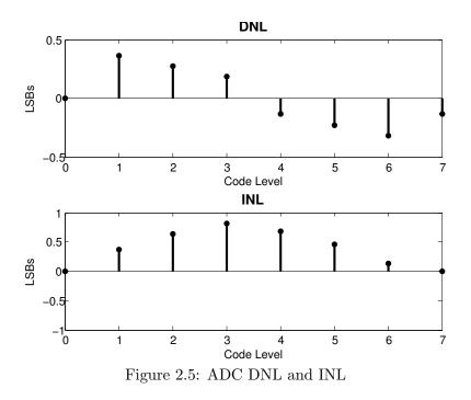
accuracy of an A/D. Using the ideal SNR Equation 2.4 the ENOB can be calculated from the measured SNDR.
