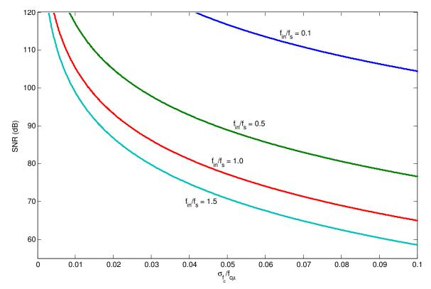
Figure 3.8: Plot of Bandwidth Mismatch for Multiple Input Frequencies
