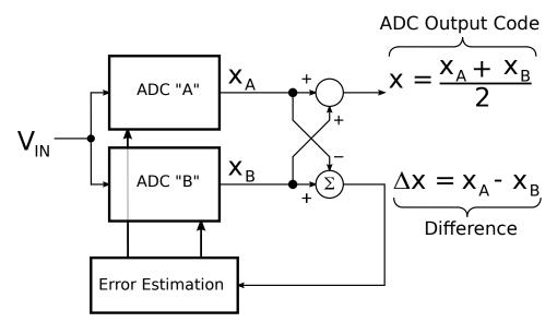
Figure 4.2: Block Diagram of Split-ADC Architecture
