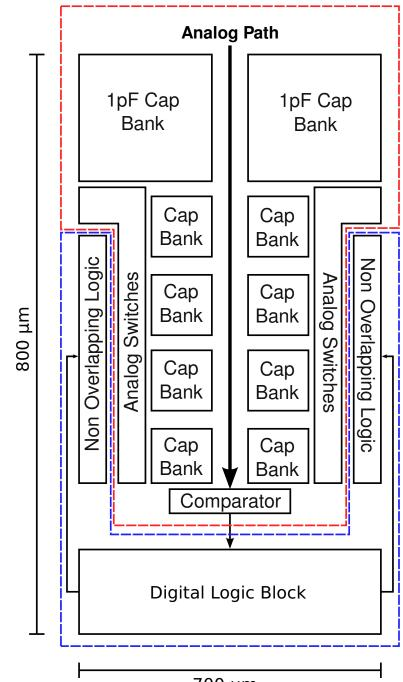
**700 μm** Figure 6.6: Split-SAR Layout Floor Plan
