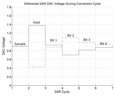
Figure 3.11: DAC Voltage Waveform of the Differential SAR
