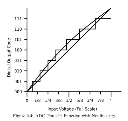
where *i* is the quantization code level [13]. For example, if the output changes levels when the analog input increases by only 3/4 LSB, then the DNL for that transition is -1/4 LSB. Each transition has an associated DNL value that can be greater than or equal to -1 as seen in Equation 2.5. In the case where the DNL is -1, the transition never occurs. When the DNL exceeds +1, the quantization level is skipped completely, which results in a missing code [12, 13].
