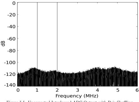
Figure 5.5: Uncorrected Interleaved ADC Output with Pair Shuffling
