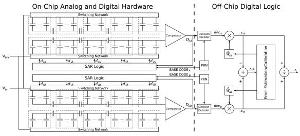
Figure 6.1: Split-SAR Block Diagram
