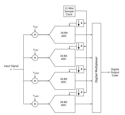
Figure 3.2: Block Diagram of 4:1 Time Interleaved Converter with Offset Error Introduced
