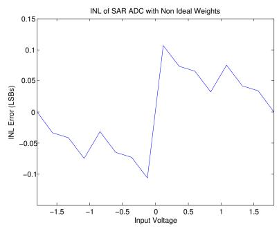
Figure 3.13: INL of Non-Ideal SAR Converter
