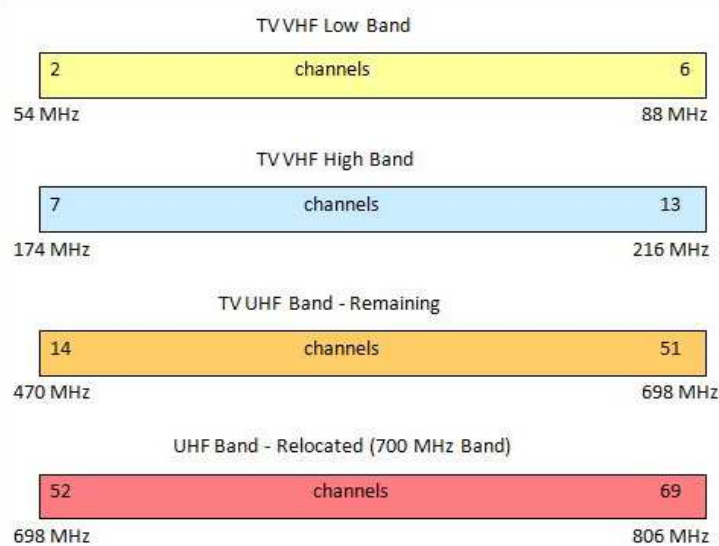
Figure 2 VHF low band and high band, and UHF Channels used for TV Broadcast Service
