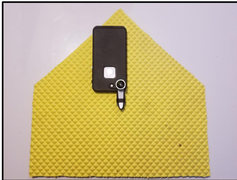
Figure 13: Setup of smartphone with fisheye lens with foam baseball plate for reference.
