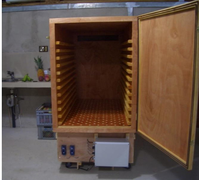
Figure 3. Front view of NTB's fruit dryer (Bertsch et al., 2015)
