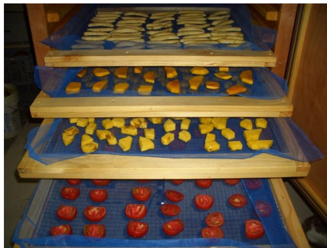
Figure 4. Wooden pallets with mosquito netting (Bertsch et al., 2015)
