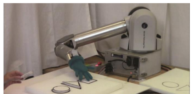
Figure 9 An arm with six degrees of freedom indicating objects on a table
