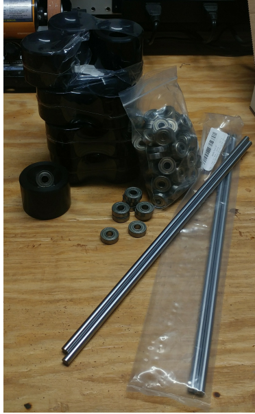
Figure 17: Omni wheel Parts
