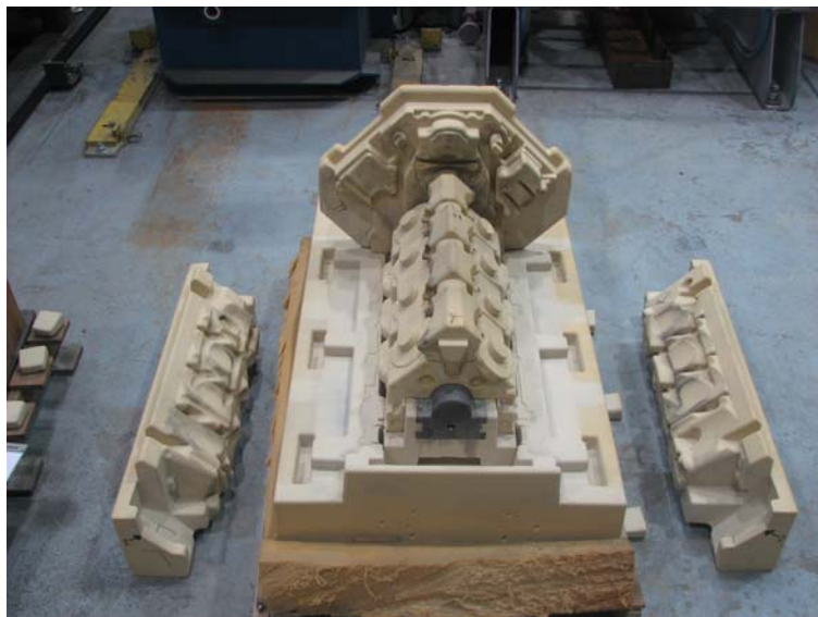
Figure 1.1: Partially disassembled core package for an eight-cylinder, v-block engine
