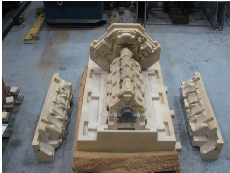
Figure 4.12: Partially disassembled engine block mold
