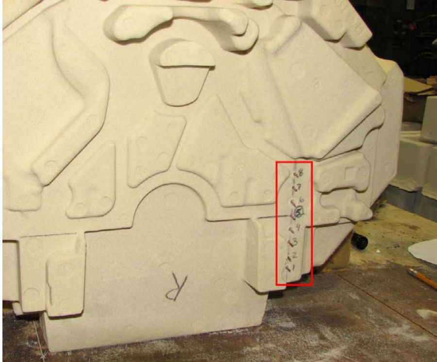
Figure 4.14: Vertical arrangement of contact probes along interior of end core
