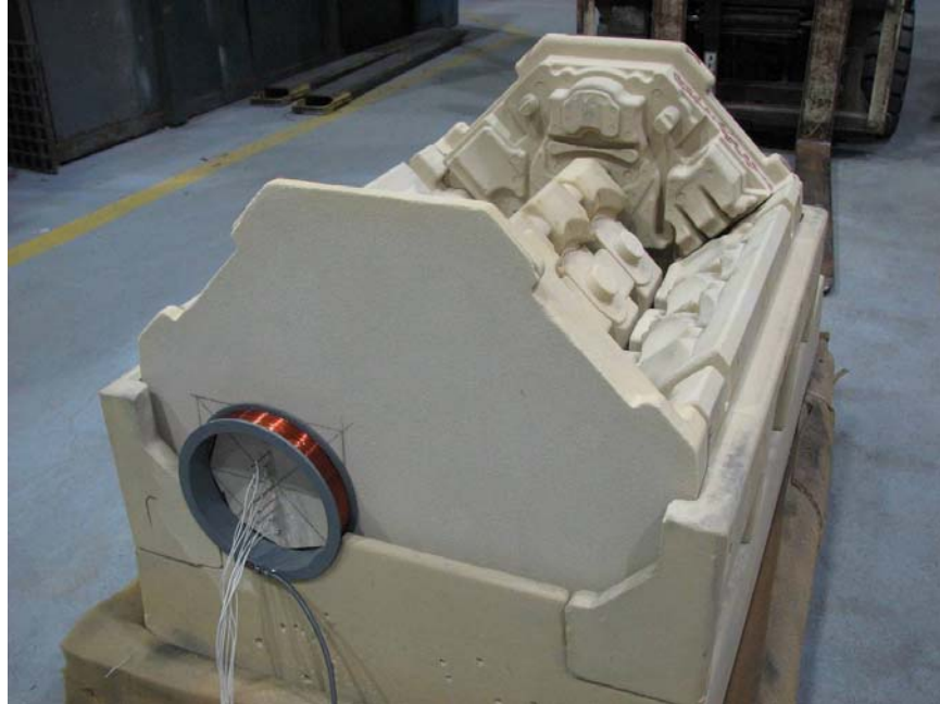
Figure 4.15: Placement of coil sensor on the exterior of the core package
