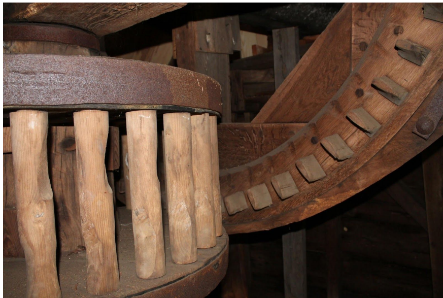
Figure 2.3.4 Wallower (left) and Brake Wheel (right) (Campbell, 2019)
