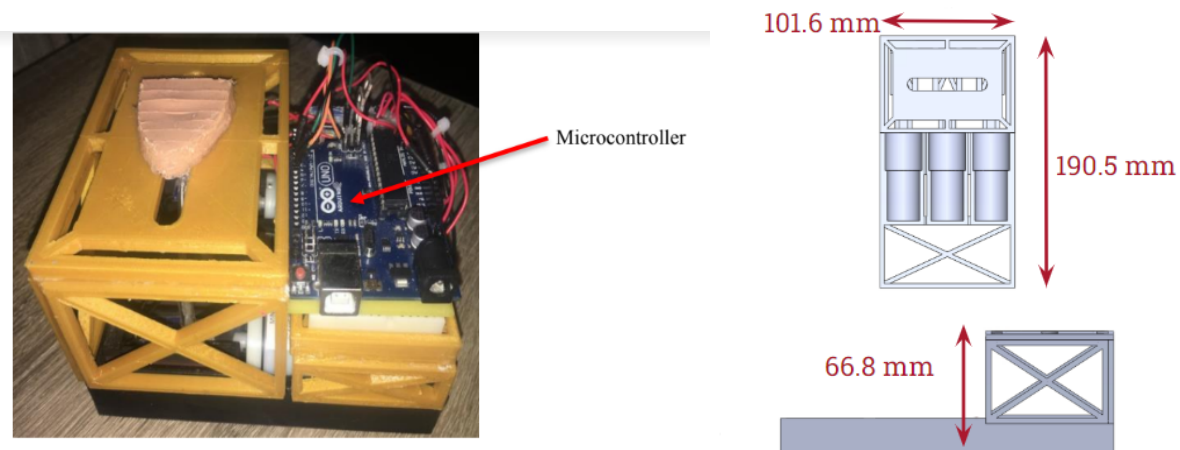
Figure 1.3: Control Module, microcontroller, and prosthetic tongue. The red arrow points to the microcontroller. The dimensions of the control module are on the right. Both as reproduced from [5]
