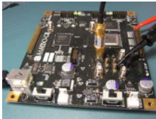
Figure 2.5: Example Setup on Sasebo-GII FPGA
