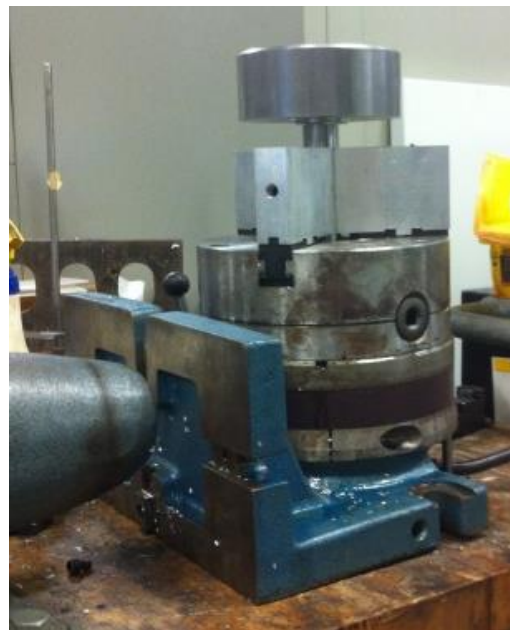
Figure 54: Three Jaw Rotary Chuck Fixture for Crankshaft Milling
