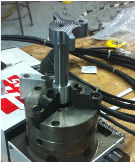
Figure 56: Rotary Fixture with Clamp Collar for 4th Axis Milling
