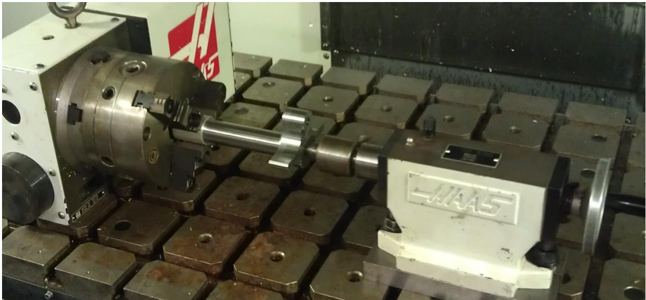
Figure 29: Crank-Shaft Fixtured for 4th Axis Machining
