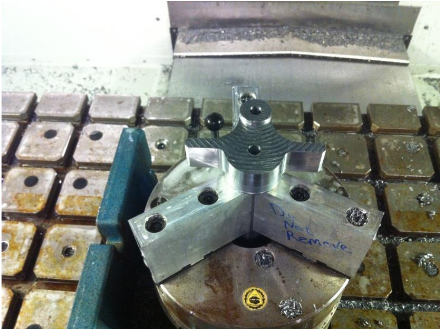
Figure 55: Crankshaft Profile Milling
