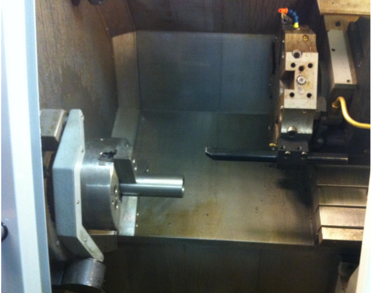
Figure 61: Sleeve ID boring with 1.5" Boring Bar
