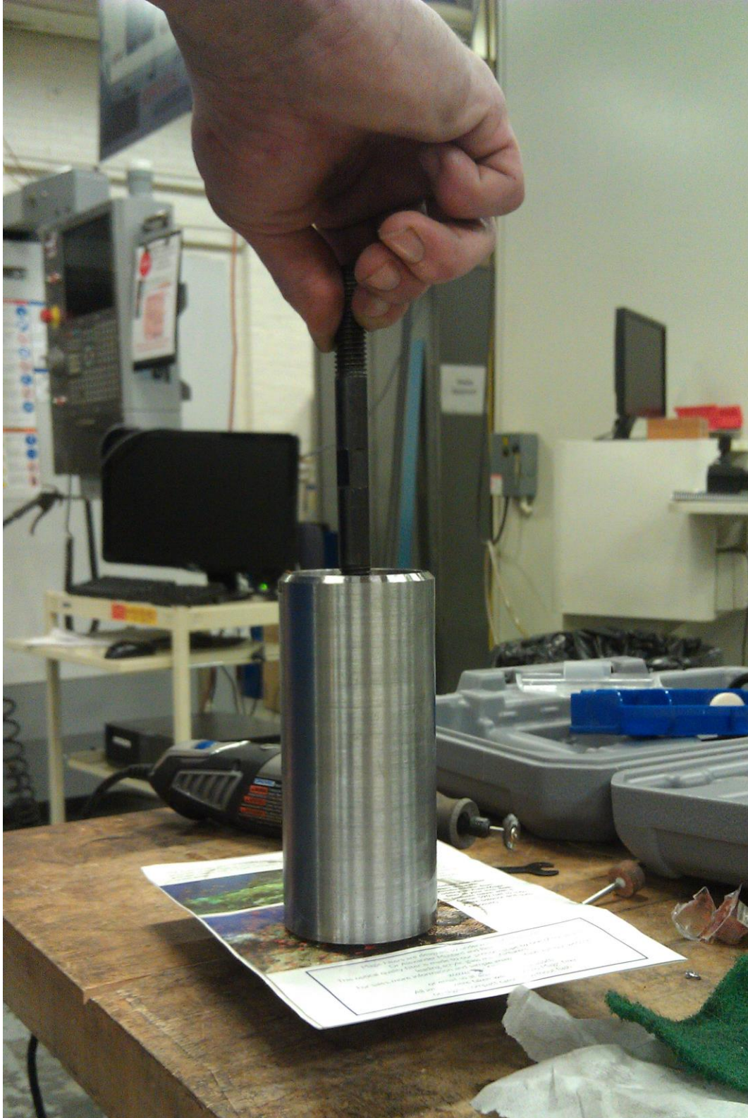
Figure 62: Piston inside Sleeve Demonstrating Airtight Seal
