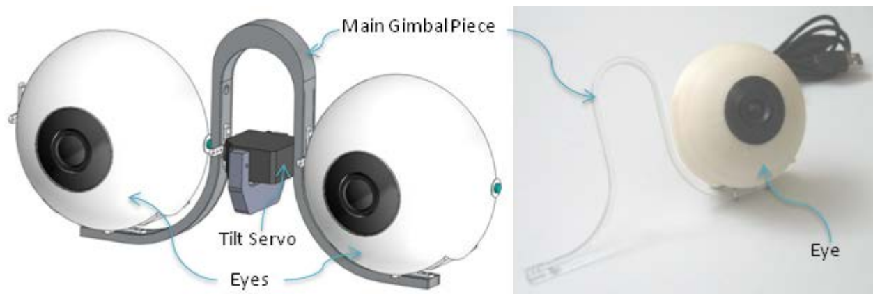
Figure 7 First Complete Design and Prototype of the Eye Mechanism
