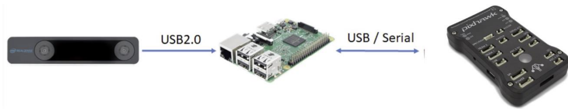
Figure 25 Intel T65 Tracking Camera to Pixhawk [9].
