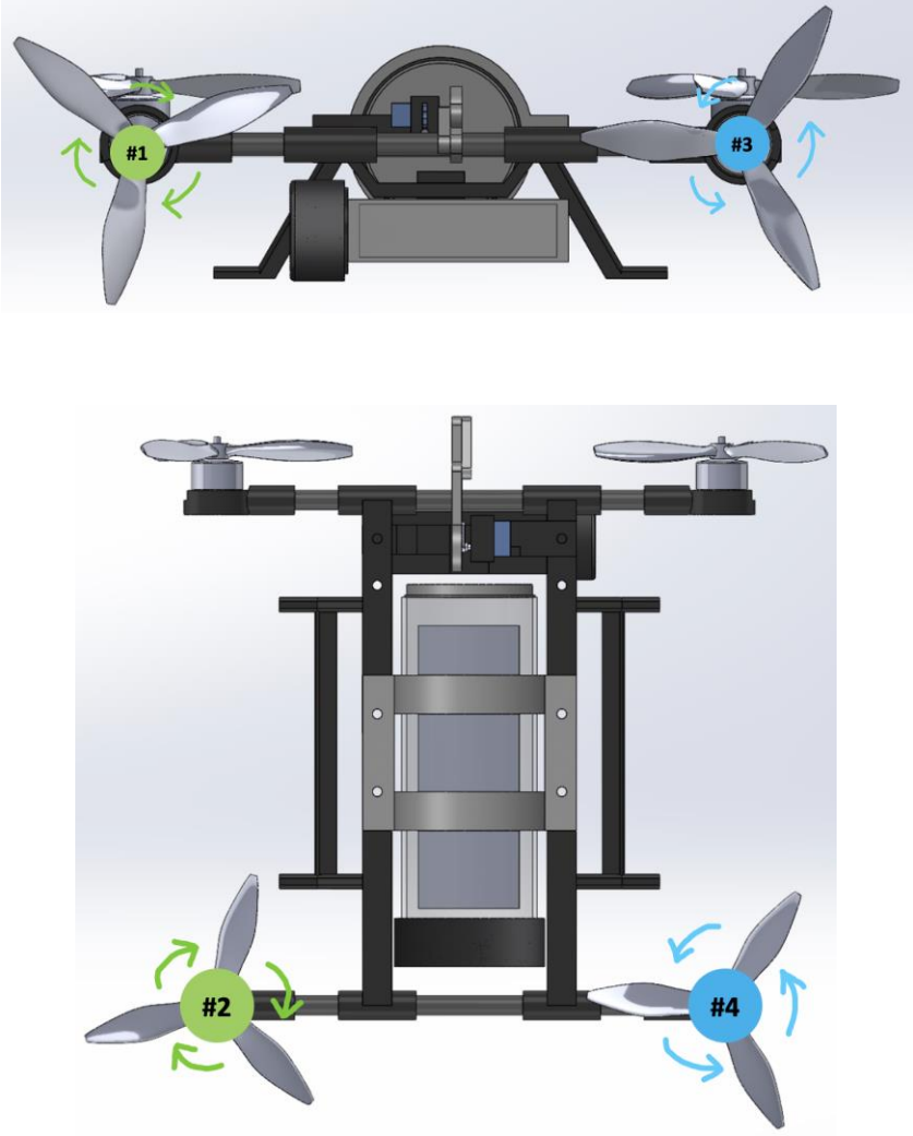
Figure 15: Direction of AUV's motor spin during underwater flight.
