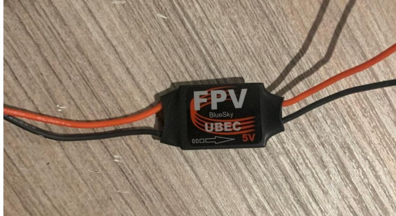
Figure 22: UBEC Power Step-Down.
