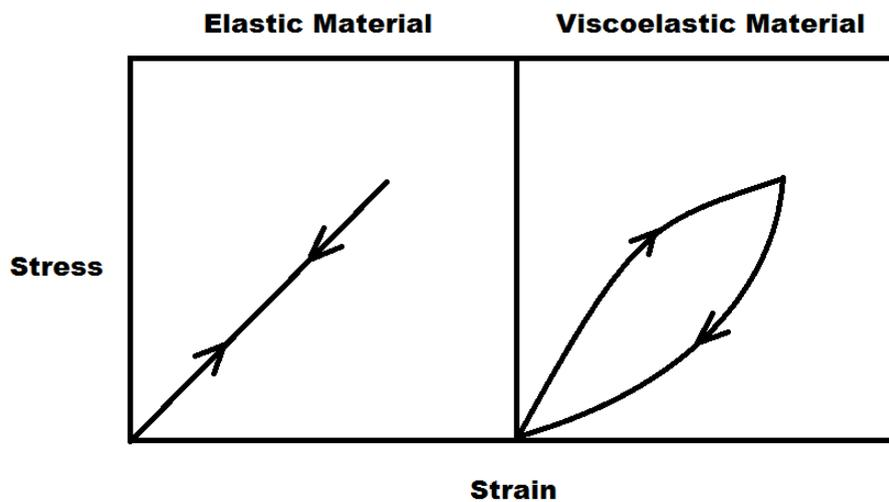
FIGURE 1.2: Stress vs Strain plot of elastic and viscoelastic materials
