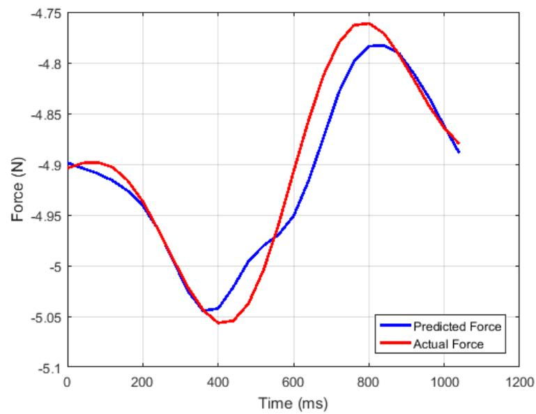
FIGURE 4.4: Plot of actual force exerted by the Hydro Muscle and the predicted force vs time
