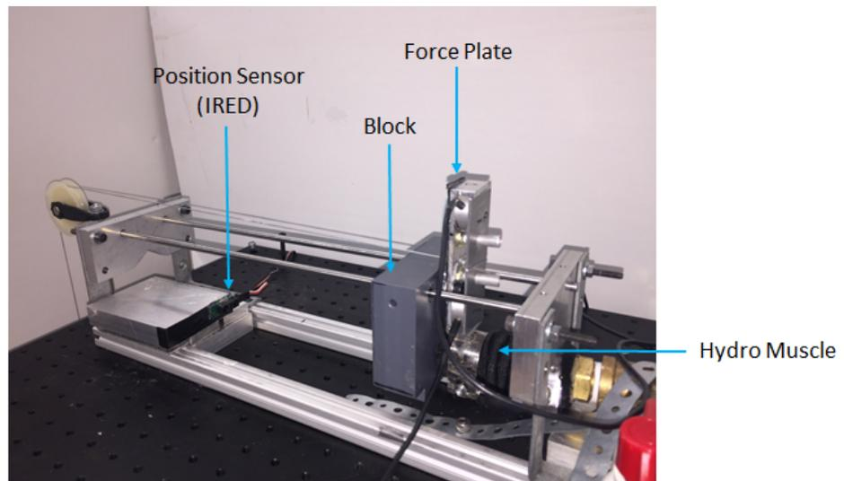
FIGURE 4.2: Final experimental setup for developing the dynamic viscoelastic model
