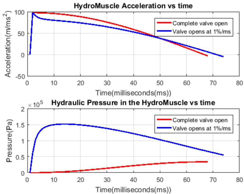
FIGURE 2.3: Mathematical model simulation of acceleration and pressure of a Hydro Muscle during relaxation
