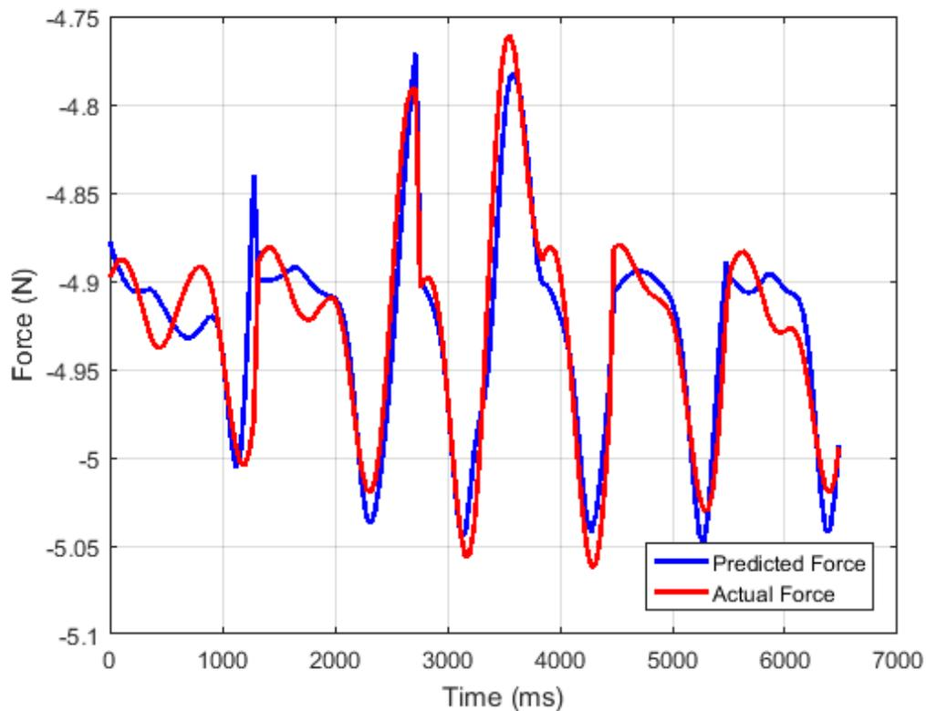
FIGURE 5.3: Plot of actual force exerted by the Hydro Muscle and the predicted force vs time for Model Validation
