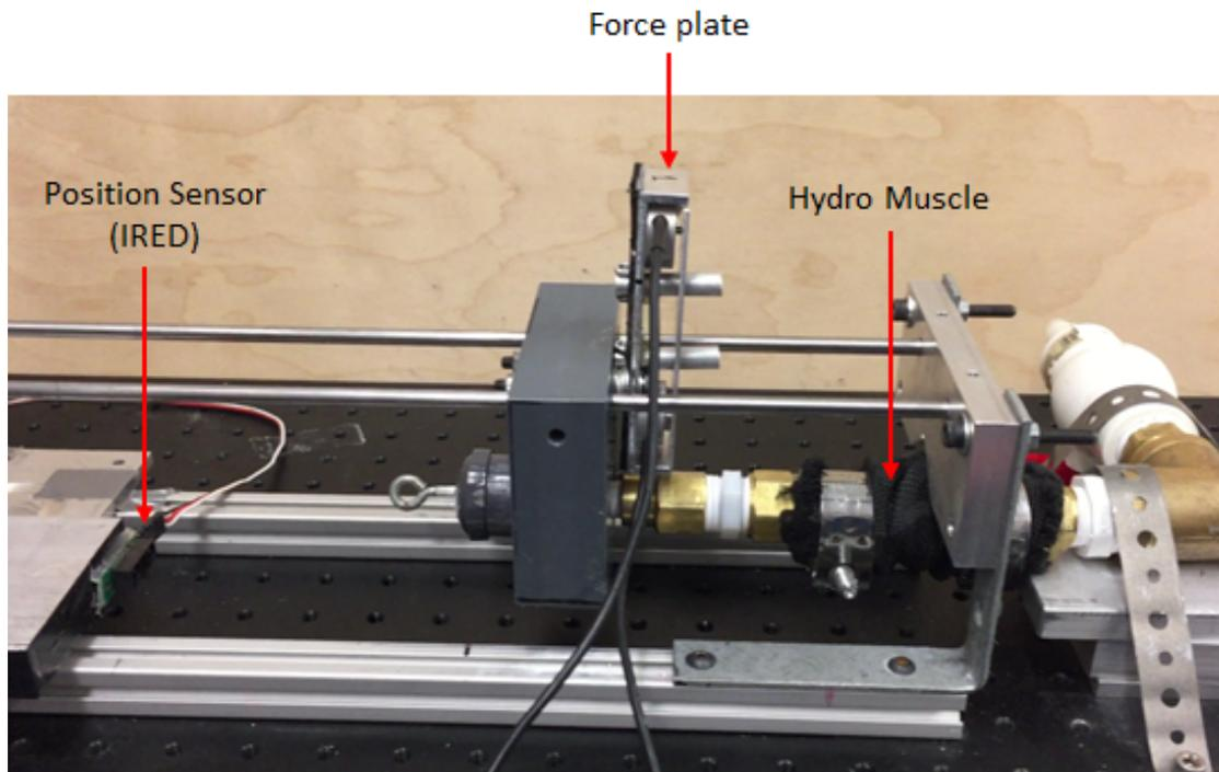
FIGURE 4.1: Experimental setup for developing the dynamic viscoelastic model
