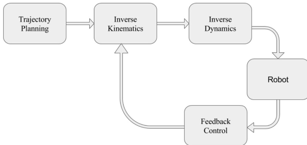
FIGURE 1.3: Feed-forward Control system using inverse dynamic model for control
