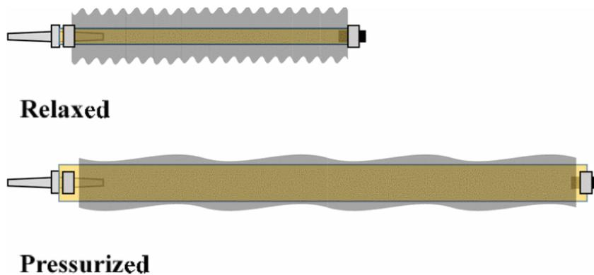
FIGURE 1.1: Hydro Muscle sketch when pressurized and relaxed
