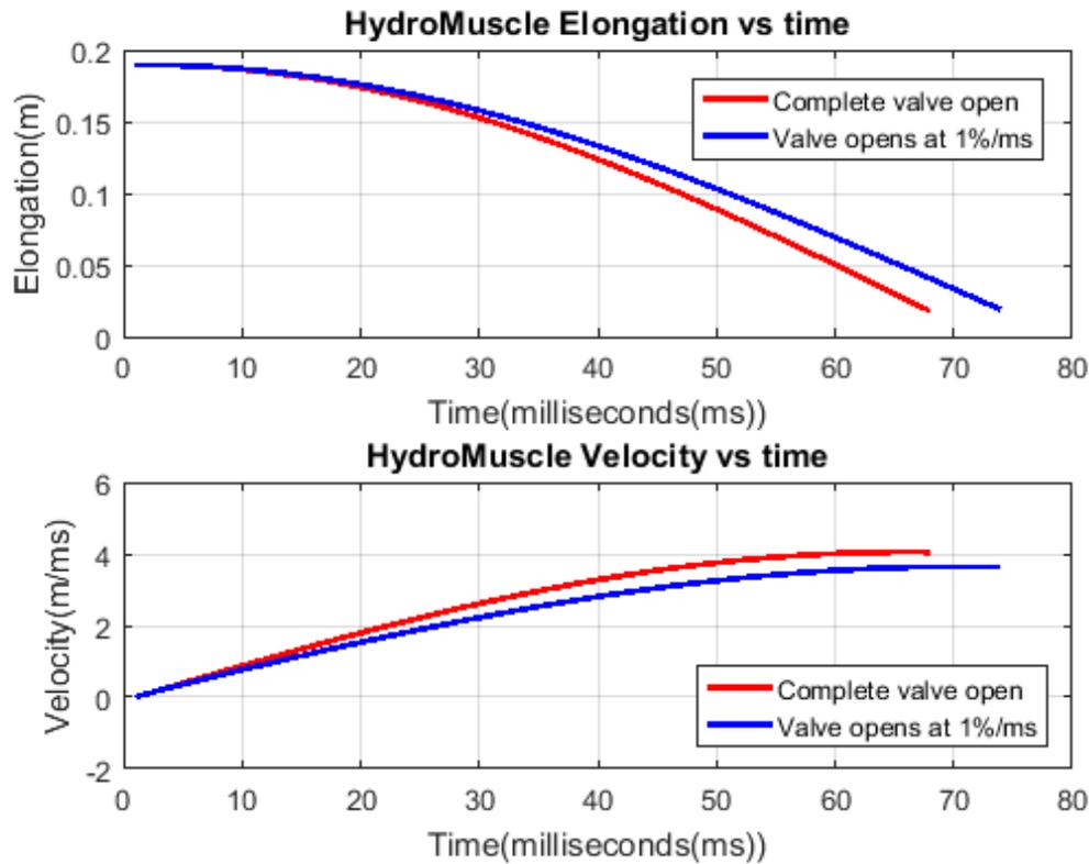
FIGURE 2.2: Mathematical model simulation of elongation and velocity of a Hydro Muscle during relaxation
