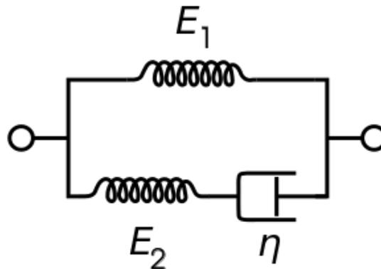
FIGURE 3.1: Standard Linear Solid Model as a combination of ideal elastic springs and viscous dash-pots
