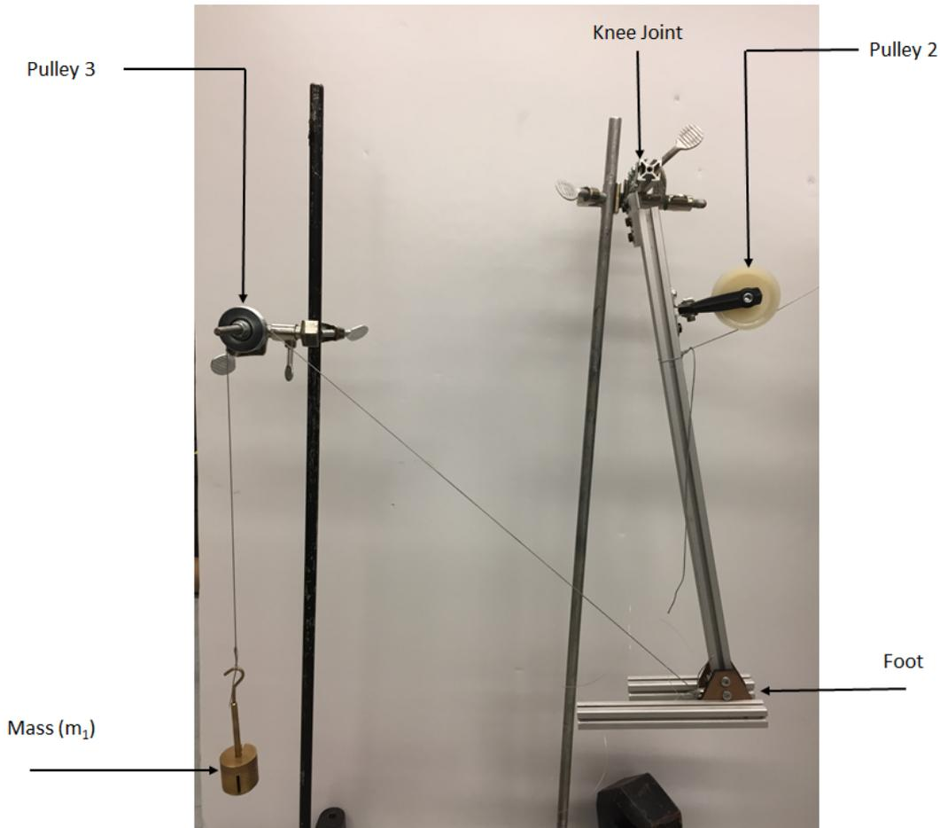
FIGURE 5.1: Experimental setup for Model Validation
