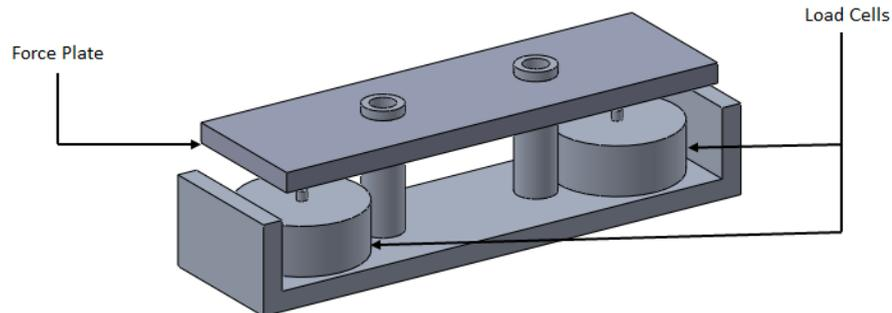
FIGURE 4.3: Custom designed force plate assembly
