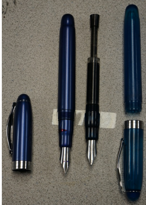
Figure 7: On the right, the body of the pen is removed to show the internal reservoir. The pen on the left has been converted. The internal reservoir was removed and the entire body acts as a reservoir instead.
