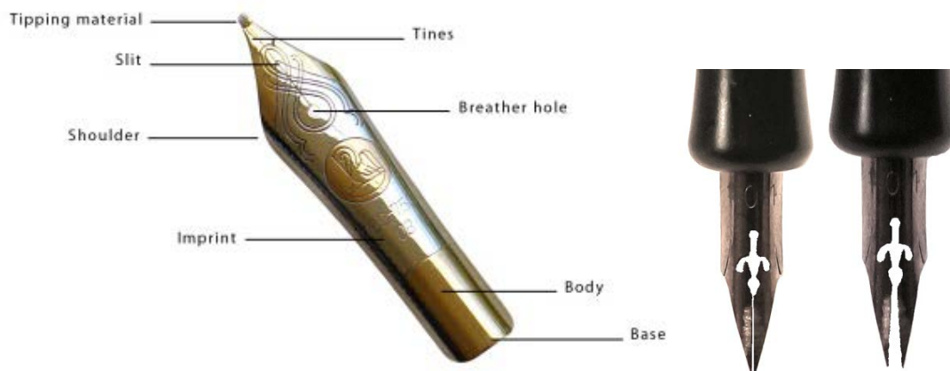
Figure 3:[LEFT] A labeled anatomy of a typical pen nib. [9] The ink flows down the slit to the tip of the pen. [RIGHT] The tines on a relaxed pen nib are nearly touching, which will create a thin line. When the nib is pressed against a writing surface, the tines spread apart which will draw a thicker line. If they spread too far apart, the capillary action will be broken and the ink will not be able to flow.
