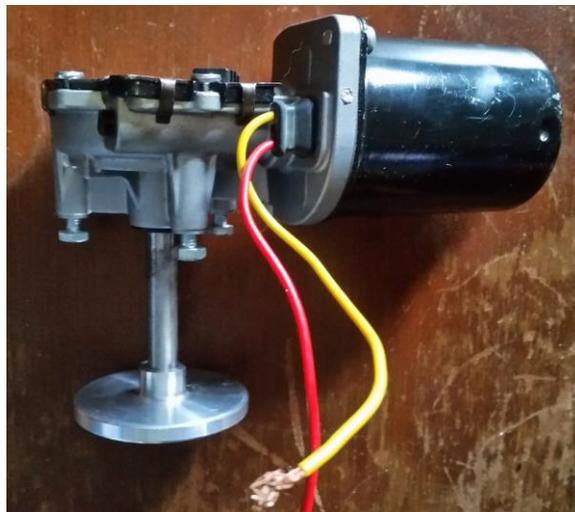
Figure 18: Cam Attached to Motor
