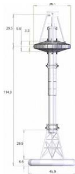
Figure 3: Point Absorber Device (Voorhis, 2012)
