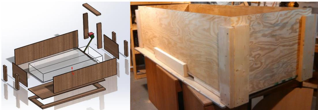
Figure 27: Exploded View and Final Construction of the Wave Tank
