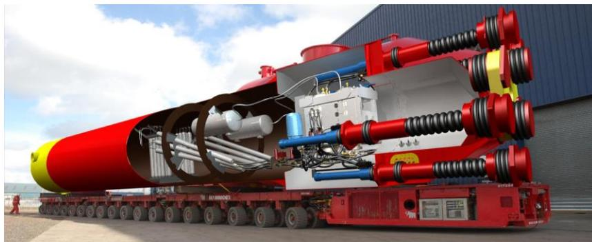
Figure 4: Wave Attenuator Device (Pelamis, 2012)
