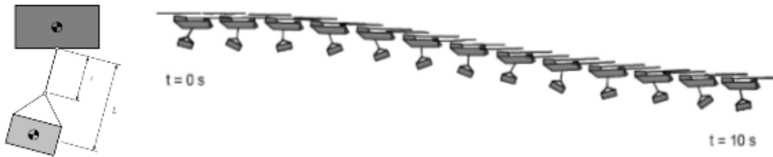
Figure 13. Simplified pendulum model of sling load (left) and animation of helicopter and load motion (right) [26, 39]
