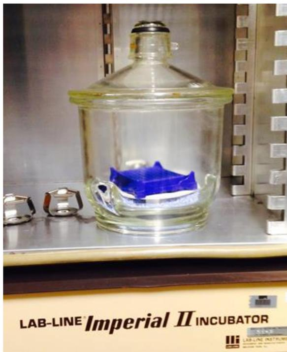
*Figure 8: Desiccator placed in incubator set to 25° C.*
