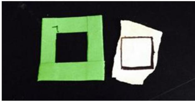
*Figure 9: 1 cm<sup>2</sup> mat used to trace known area on inner surface of eggshell.*
