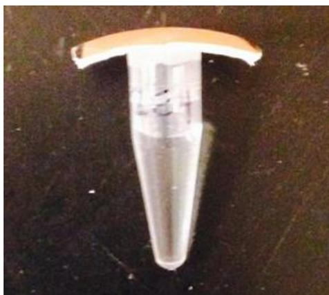
**Figure 7: Eggshell super-glued to top of a 0.25 mL microfuge tube.**
