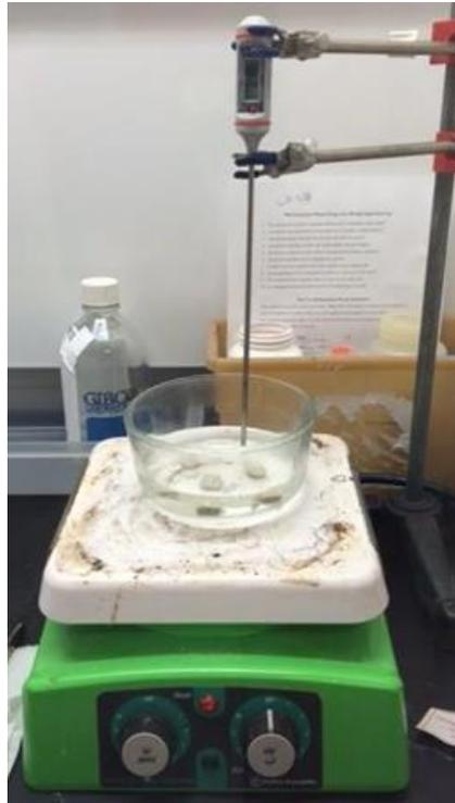
***Figure 5: Apparatus for removing membranes from COLO eggshell fragments.***
