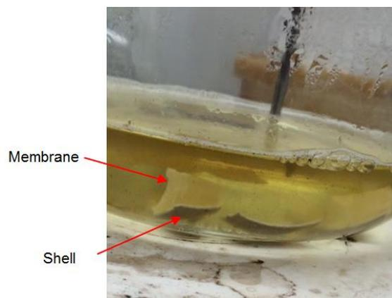
***Figure 6: Treatment with 5% NaOH for membrane removal.***
