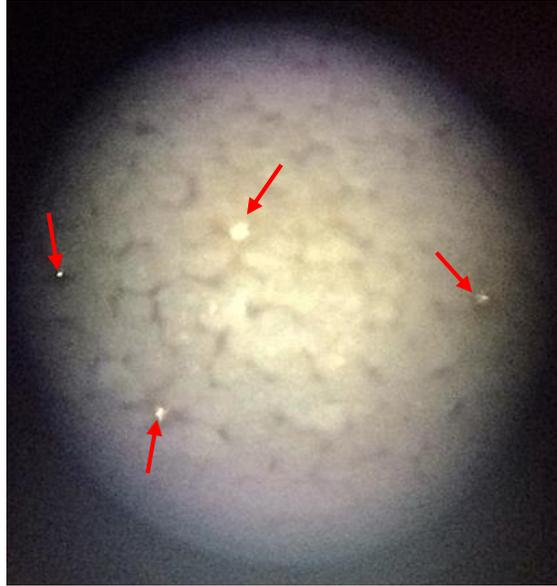
**Figure 10: Pores observed under a light microscope (50X magnification).**
