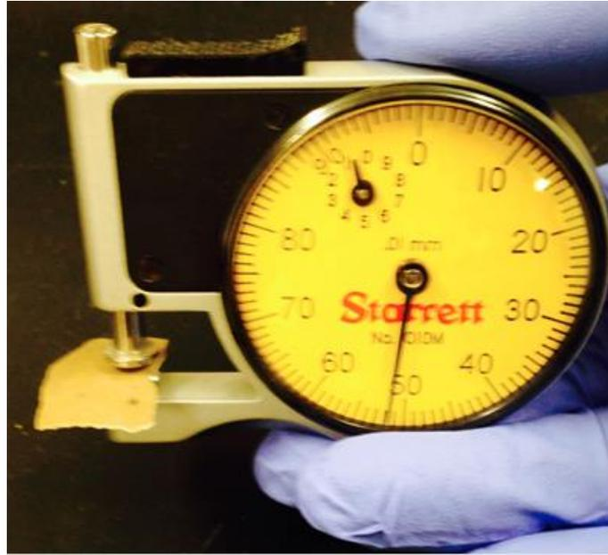
***Figure 11: Obtaining thickness measurements with a custom 1010M Starrett micrometer.***
