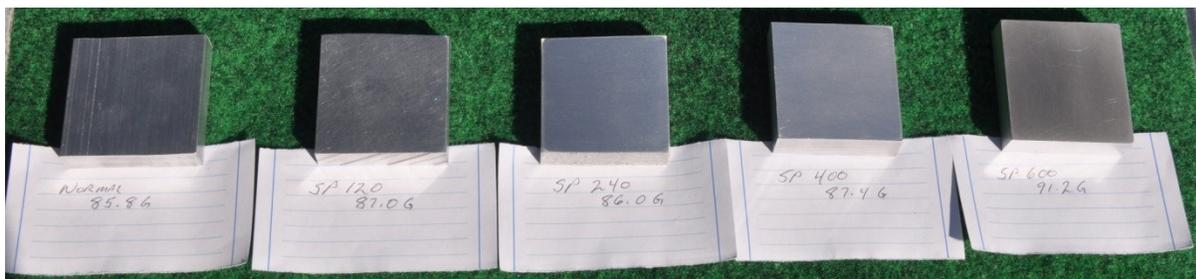
Picture 4: Test samples: Normal, SP120, SP240, SP400, SP600 respectively
