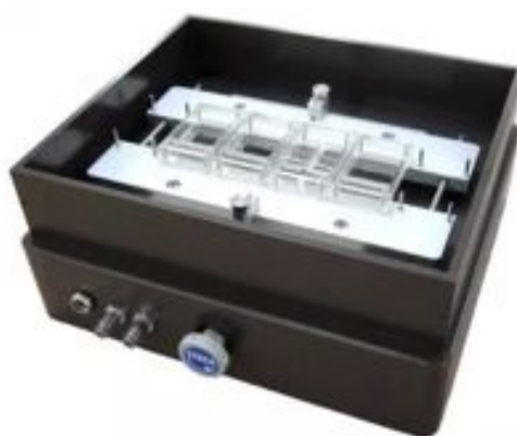
Figure 2.3: Strex STB-140 with four stretching wells loaded for uniaxial strain(Copyright © 2018 Amuza Inc.).
