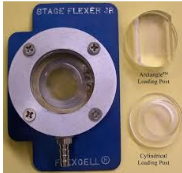
Figure A9: StageFlexer Jr. assembly and available loading posts(Copyright © 2011 Flexcell International Corporation).
