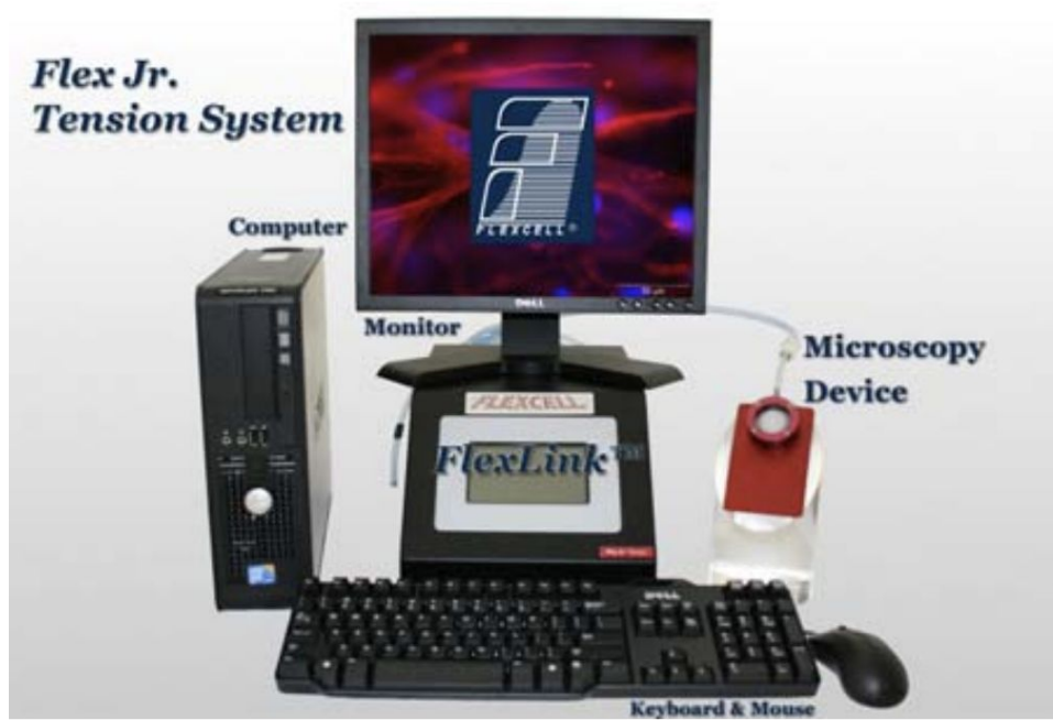
Figure A7: The complete cell stretching system using the Flex Jr. Tension System and StageFlexer microscopy device(Copyright © 2011 Flexcell International Corporation).
