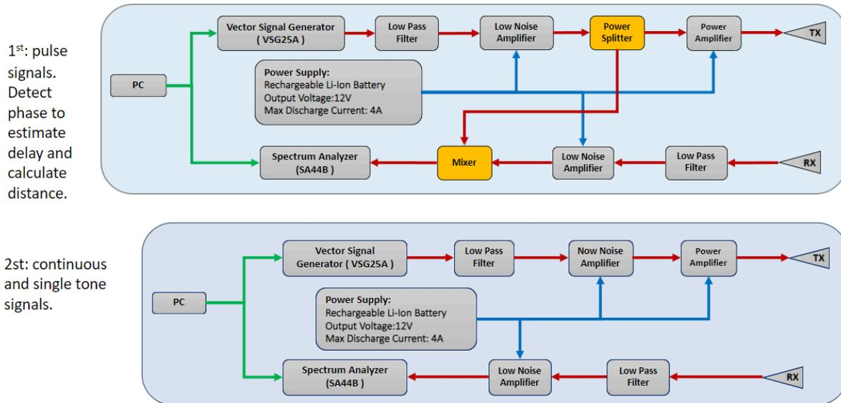
*Figure 2.1.1 SFCW Radar Configurations*
