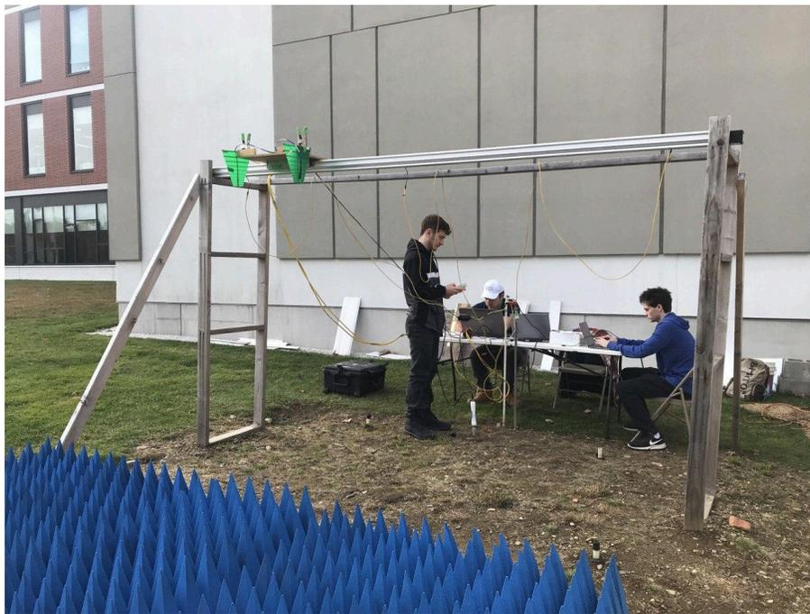
*Figure 3.3.2 Gateway Park SoilX Site Radar Measurements without observers*
