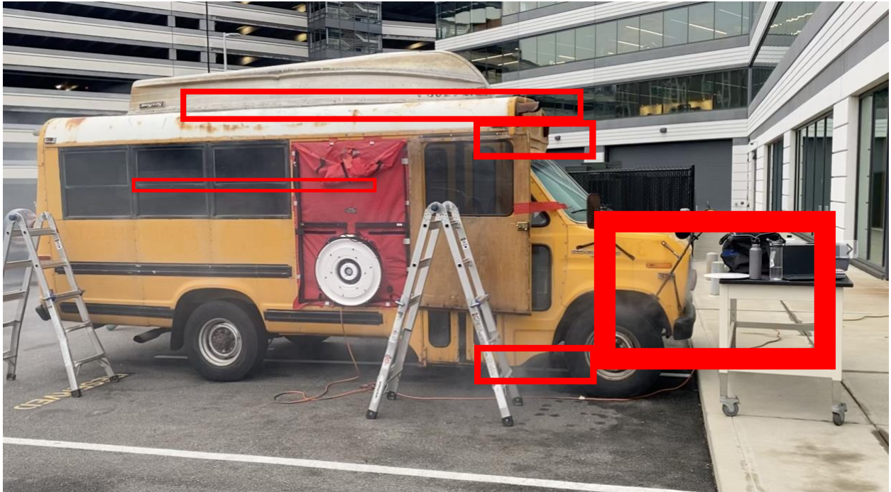
Figure 15, points of air leakage
