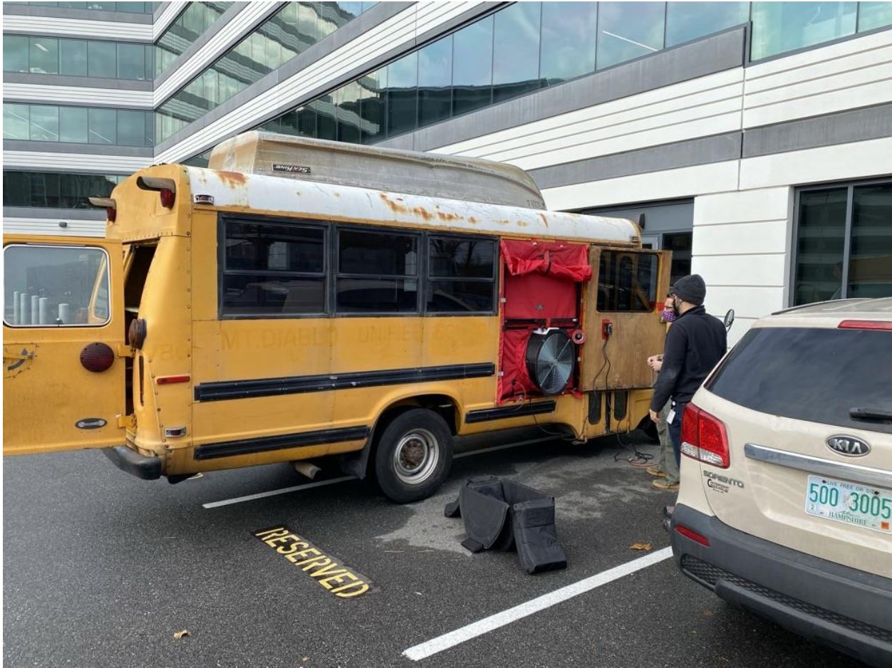
Figure 7, blower door installed for negative test
