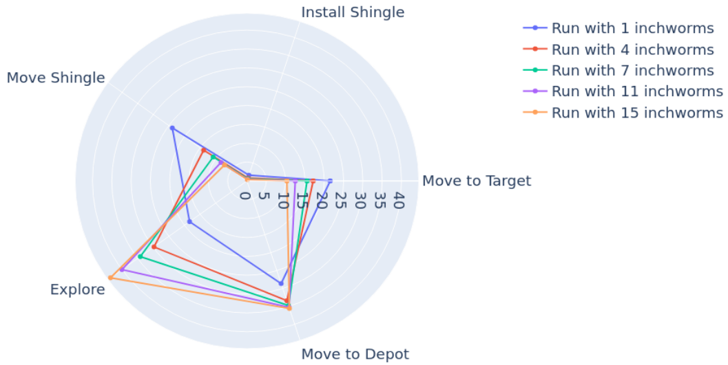
Share of Actions Taken in Run by Average Inchworm On a 30x30 roof with the Ox Plowing Pattern
