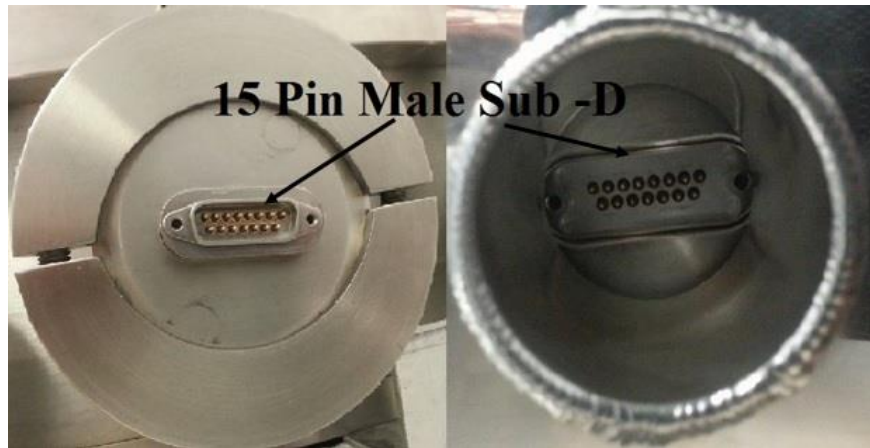
Figure 44: T4’s 15-Pin Double Sided Sub-D Feedthrough, outside (left) and inside (right)
