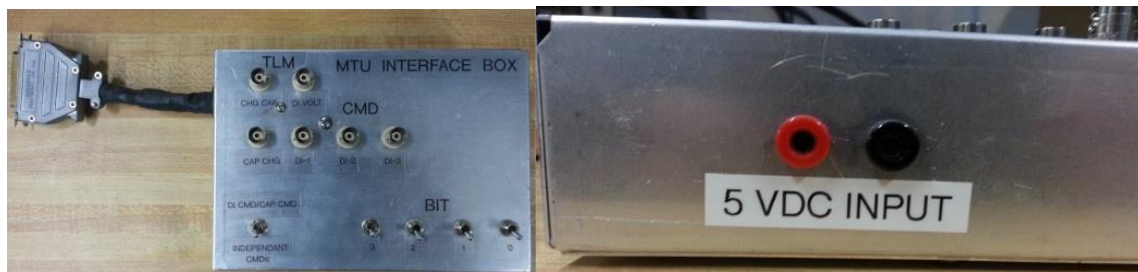
Figure 9: MTU Interface Box (left) with Power Input Connectors (right)
