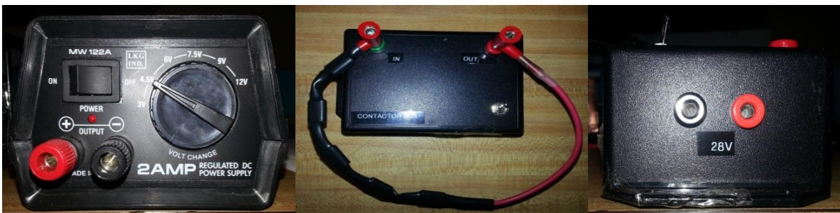
Figure 10: Power Supply (left) and Contactor Box (middle) with Power Input (right)
