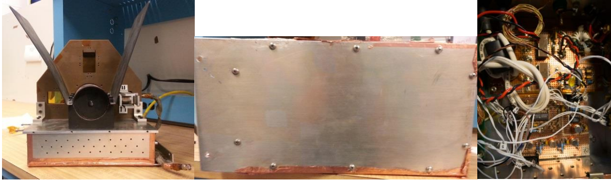
Figure 7: Back of MTU (left), Bottom Access Panel (middle) and Inner Electronics (right)
