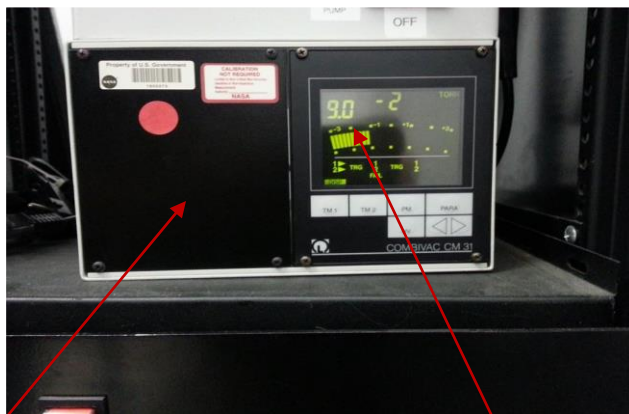
Figure 36: CombiVac Displaying Chamber Pressure of 90 mTorr (11/08/2013 @ 10:40 AM)
