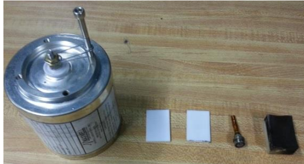
Figure 11: Capacitor, Teflon Wafers, Used Fuel Bar, and Spare Spark Plug
