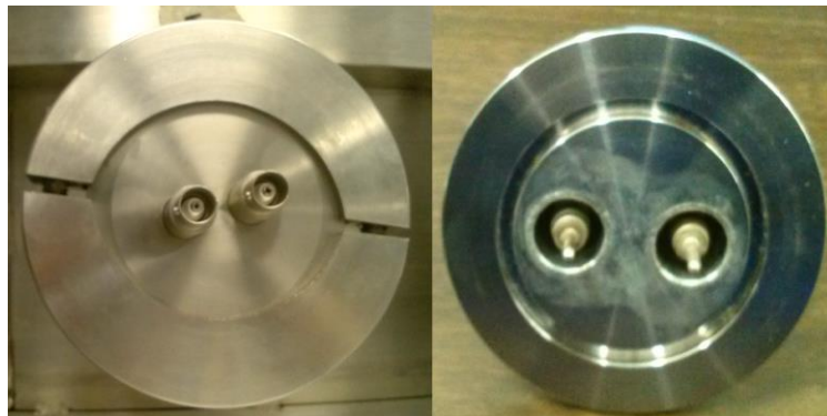
Figure 46: T4's Single Ended, Grounded Shield Coaxial Feedthrough, outside (left) and inside (right)
