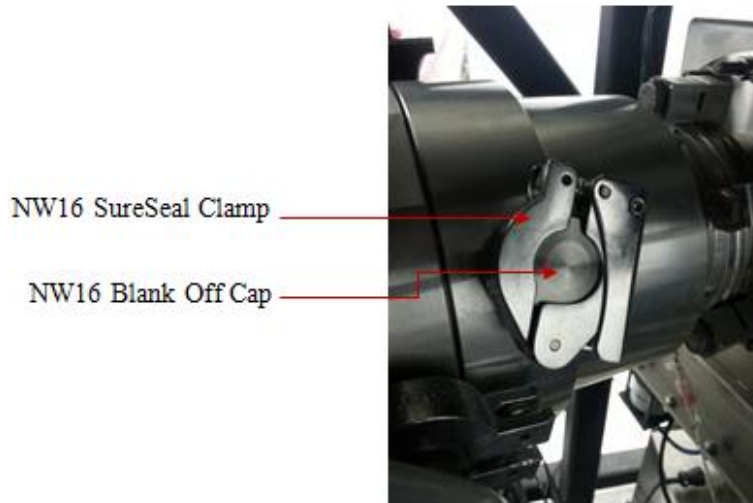
Figure 37: Turbopump Valve with Components from Nor-Cal
