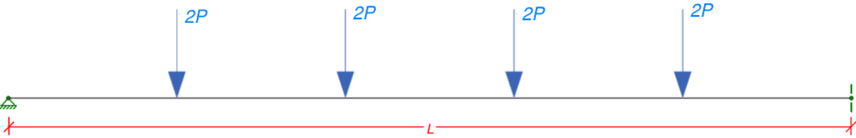
Figure 10: Sample Girder Scheme with Four Interior Purlins of Load 2P, which Indicates Purlins Sitting on Girder from Both Sides
