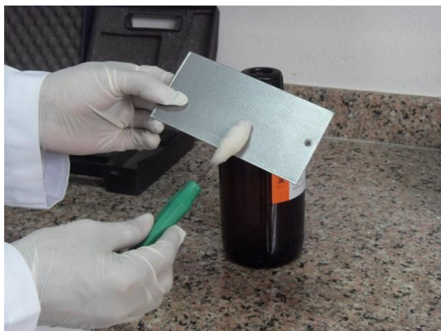
Figure 19 shows how the MEK test is performed: the MEK is applied to a Q-tip and then the Q-tip is used to rub the surface of the painted panel (Boxall and Fraunhofer, 1981).
