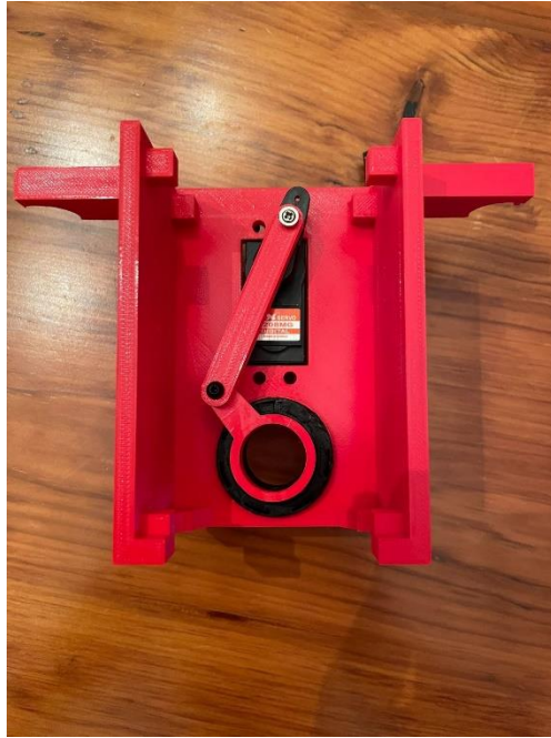
Figure 30: 3D printed model of final spray-bar mechanism
