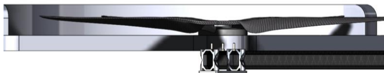
Figure 8: Side view of the initial propeller guard design
