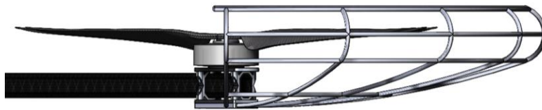
Figure 9: Side view of the modified propeller guard design
