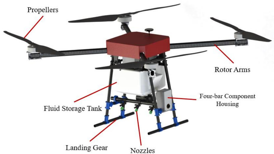
Figure 1: Drone's Mechanical Structure
