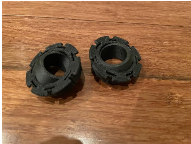
Figure 31: 3D printed customized spray-bar bearings
