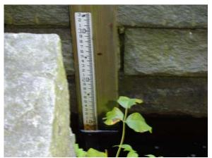
Figure 4.4. Gauging station at site MB1 at the confluence of the Wachusett Reservoir.
