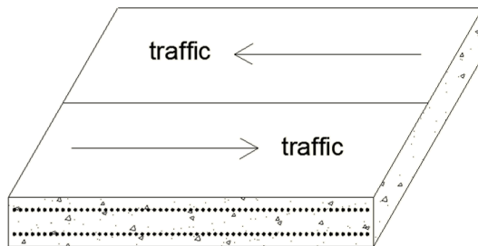
Figure 12: Direction of reinforcement bars in bridge deck (not drawn to scale)
