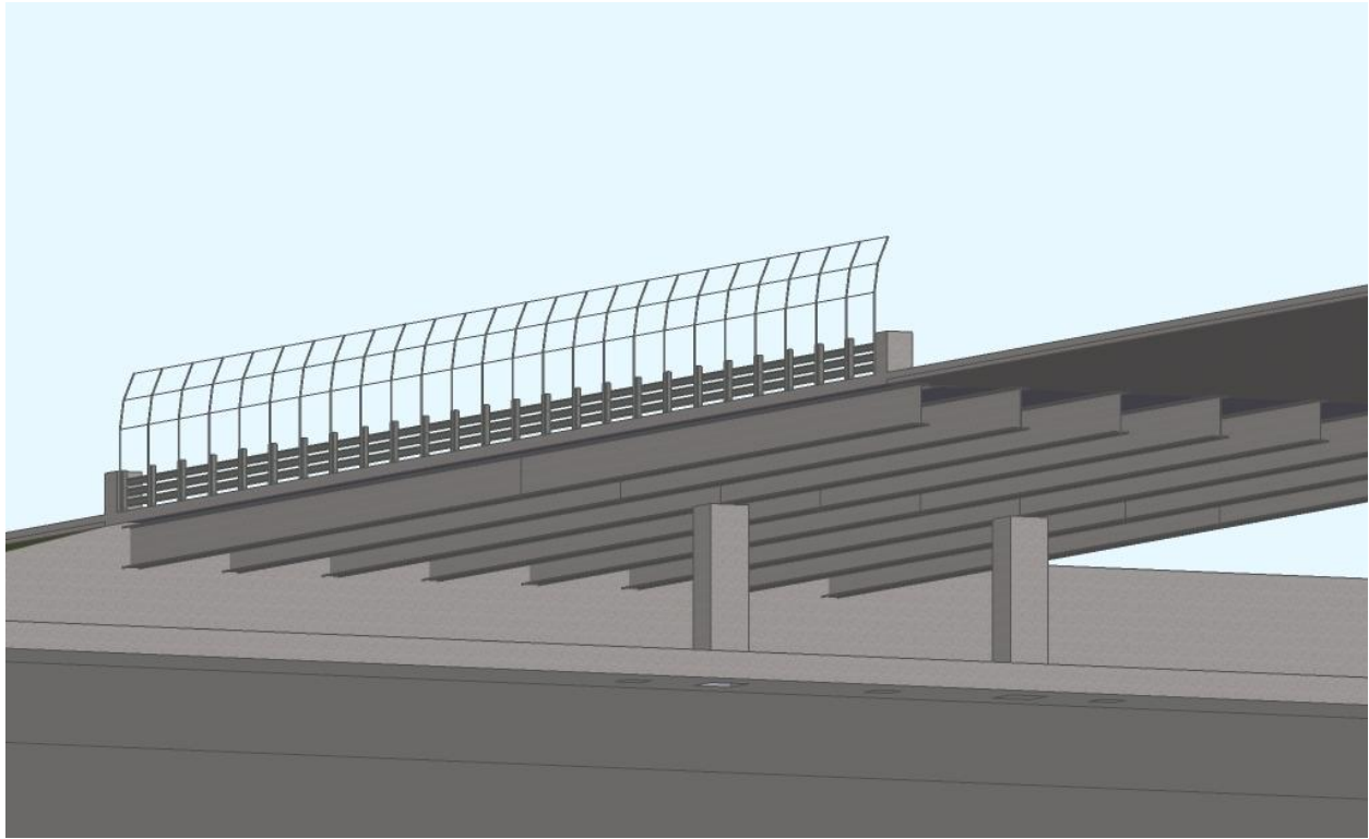
Figure 18: Proposed concrete columns and steel girders for Belmont Street/Route 9 Bridge re-design (View 1)
