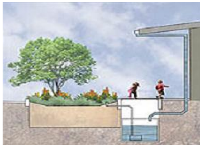
Figure 39: Rooftop Rainwater Collection System (taken from http://www.svrdesign.com/winslow_way.html )
