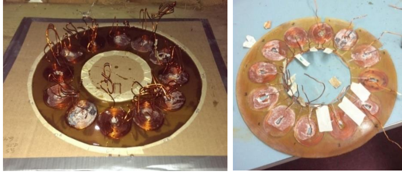
Figure 55: Stator Before and After Fiberglass Resin Pour
