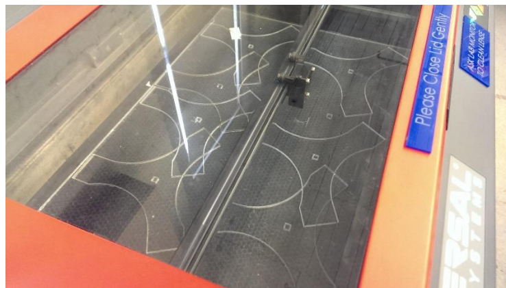
Figure 50: Laser Cut Struts for Blade Assembly
