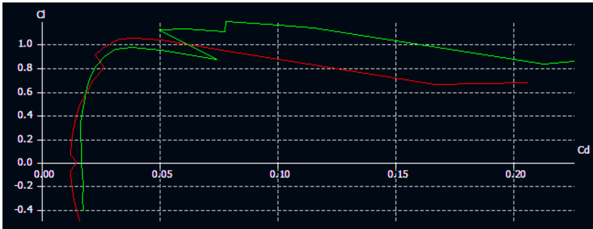
Figure 2: Simulated Profile in Comparison with NACA0012
