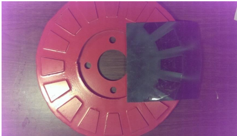
Figure 53: Magnet Rotor with Magnetic Field Paper Showing Magnetic Field
