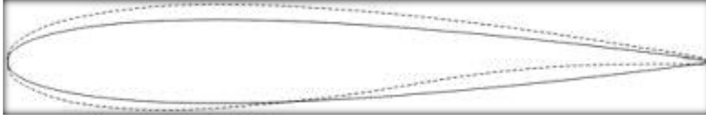
Figure 35: Comparison of Optimized Hydrofoil (NACA0012 airfoil = solid, optimized airfoil = dashed)
