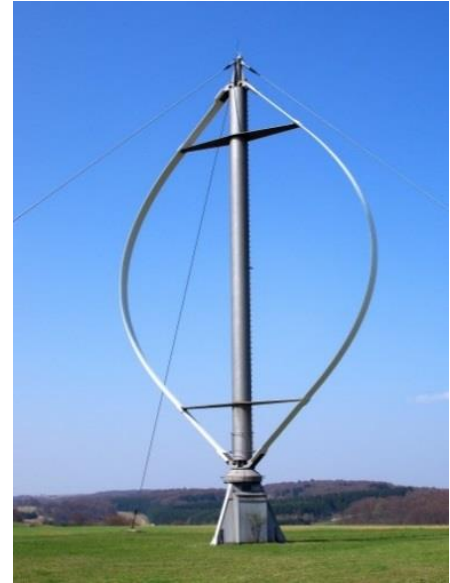
Figure 14: A Darrieus Vertical Axis Turbine (Aarchiba, 2007)
