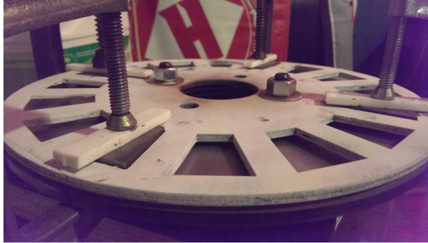
Figure 52: Assembly of a Magnet Rotor Plate
