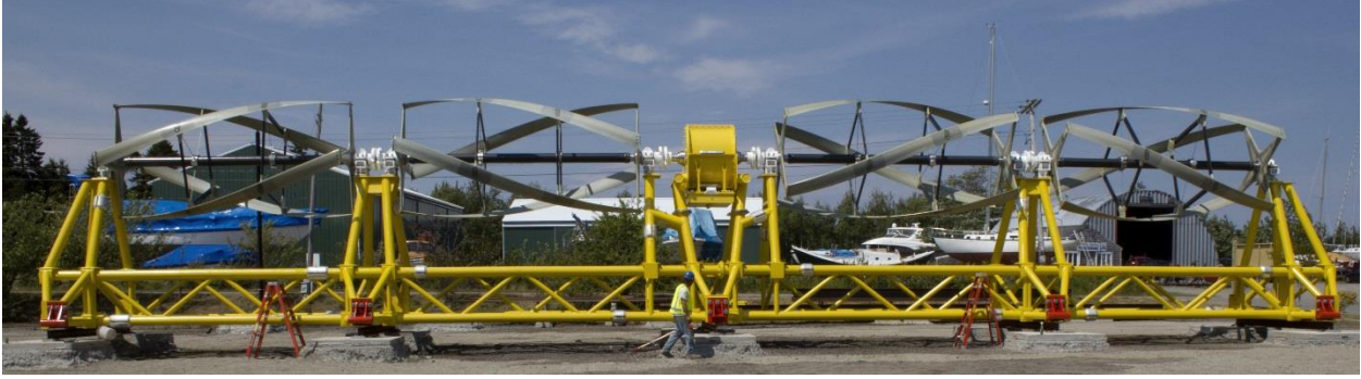
Figure 21: Ocean Renewable Power Company's Large Scale Marine Current Generator (Cobscook Bay Tidal Energy Project, 2012)
