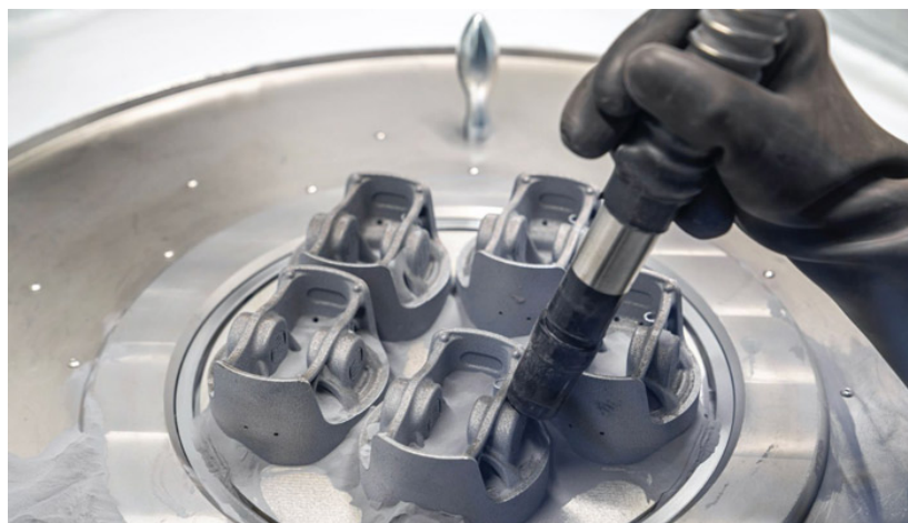
Figure 2: Excess Aluminum Powder in Piston Fabrication
