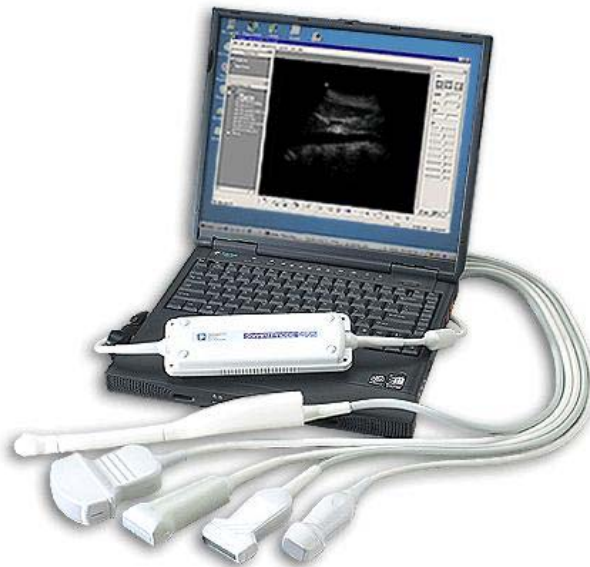
Figure 2.1: Terason 2000 ultrasound scanner system, showing the SmartProbe (on top of the laptop) and several array transducer types
