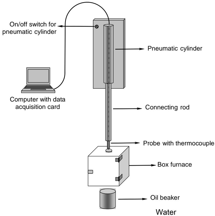
Figure 6. Quenching probe system.
