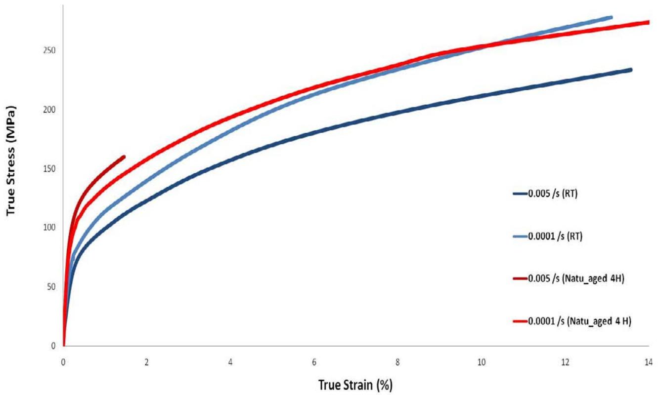
Figure 40. True stress-strain curves for supersaturated and naturally aged A356 alloy.
