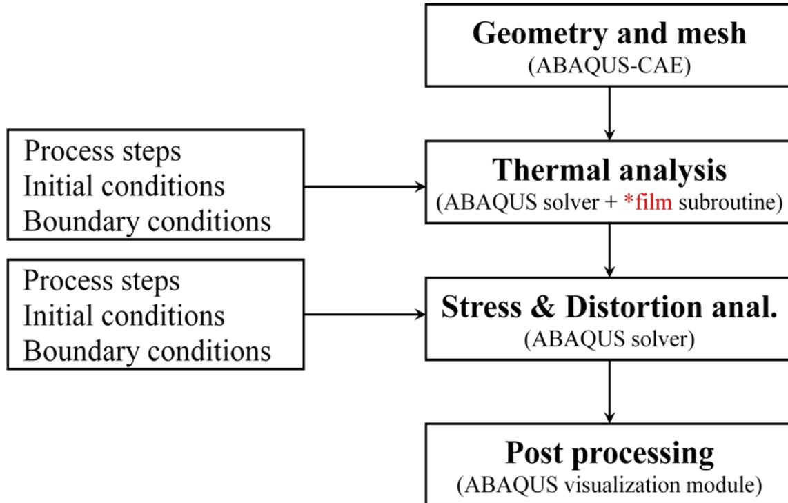
Figure 1. Solution procedures for the ABAQUS model.
