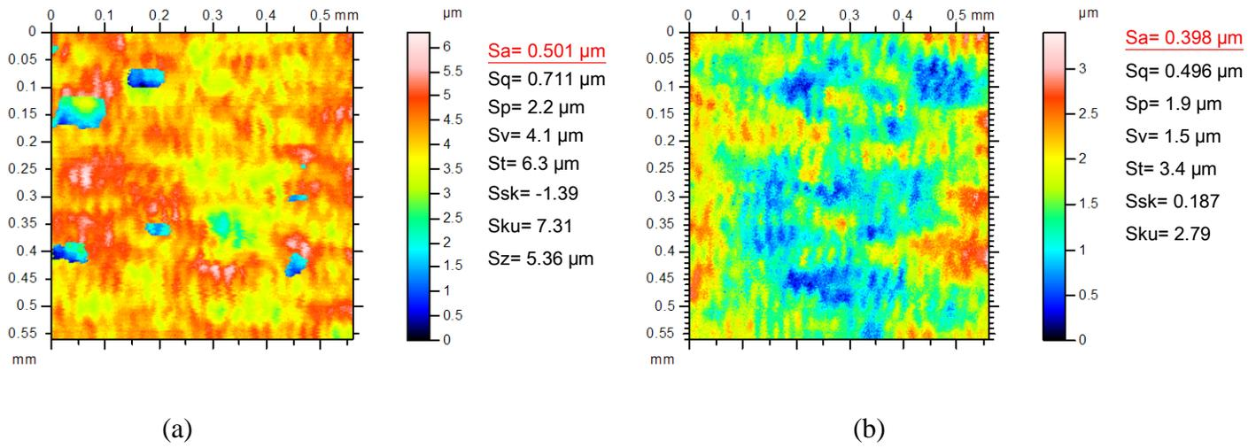
Figure 11. Measured surface roughness for (a) the cast part, and (b) the probe.
