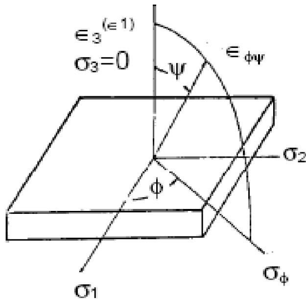
Figure 32. A schematic representation of a surface under plain stress. [14]
