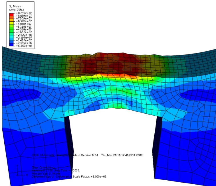
Figure 30. Thermal-stress prediction for horizontal quenching after quenching step.
