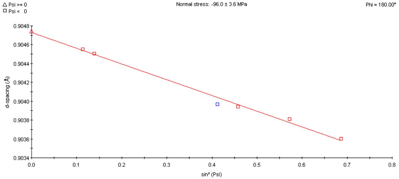
Figure 35. Change in d-spacing with  $\sin^2\psi$  for the vertically quenched part.
