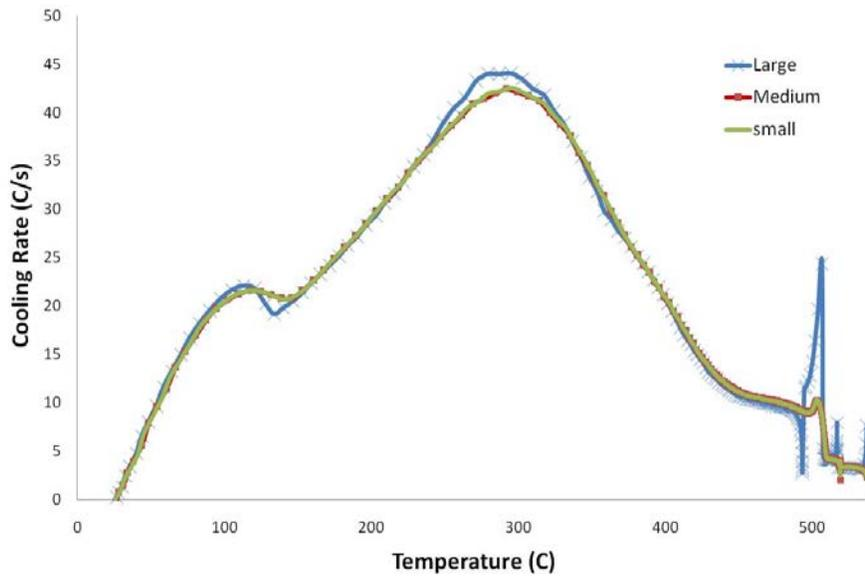
Figure 21. Cooling rates at the selected node obtained by simulation with different mesh densities.
