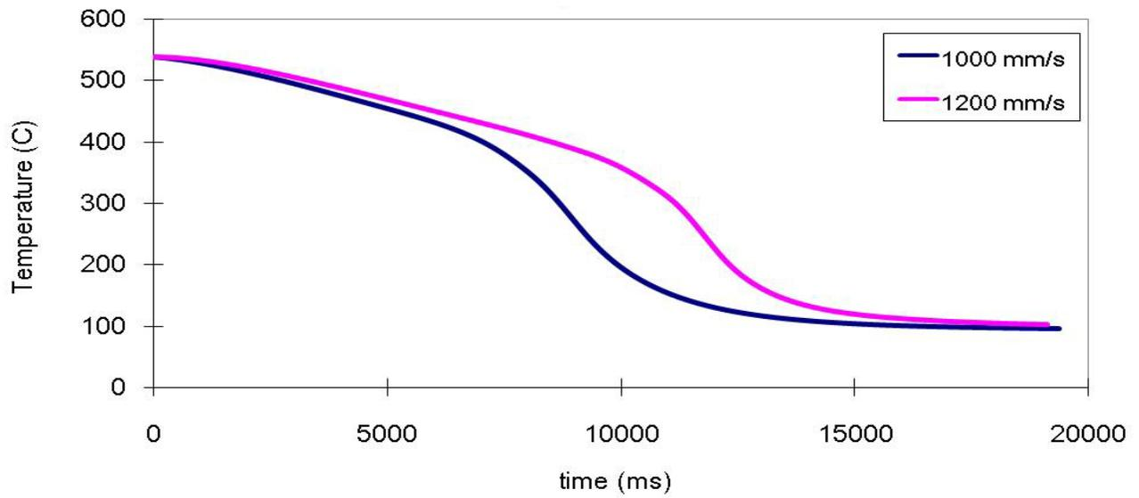
Figure 8. Measured cooling curves for A 356 alloy.
