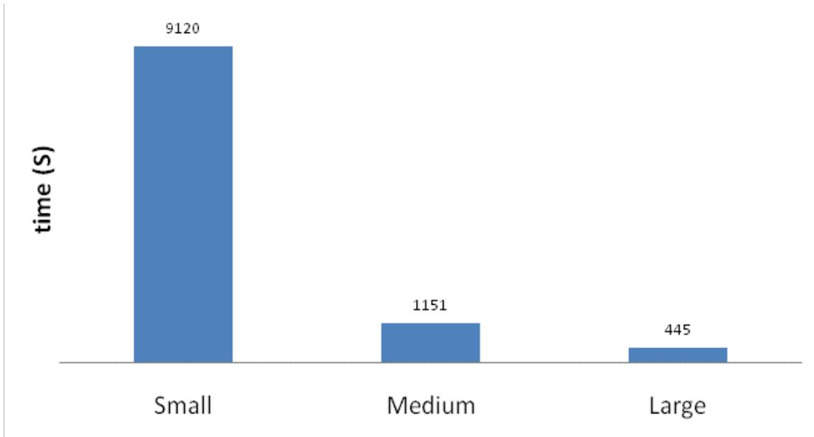
Figure 22. Computational time for the different mesh densities.
