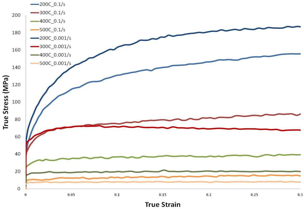
Figure 14. True stress-strain curves for supersaturated alloy at elevated temperature for strain rates = 0.001/s and 0.1/s. [10]
