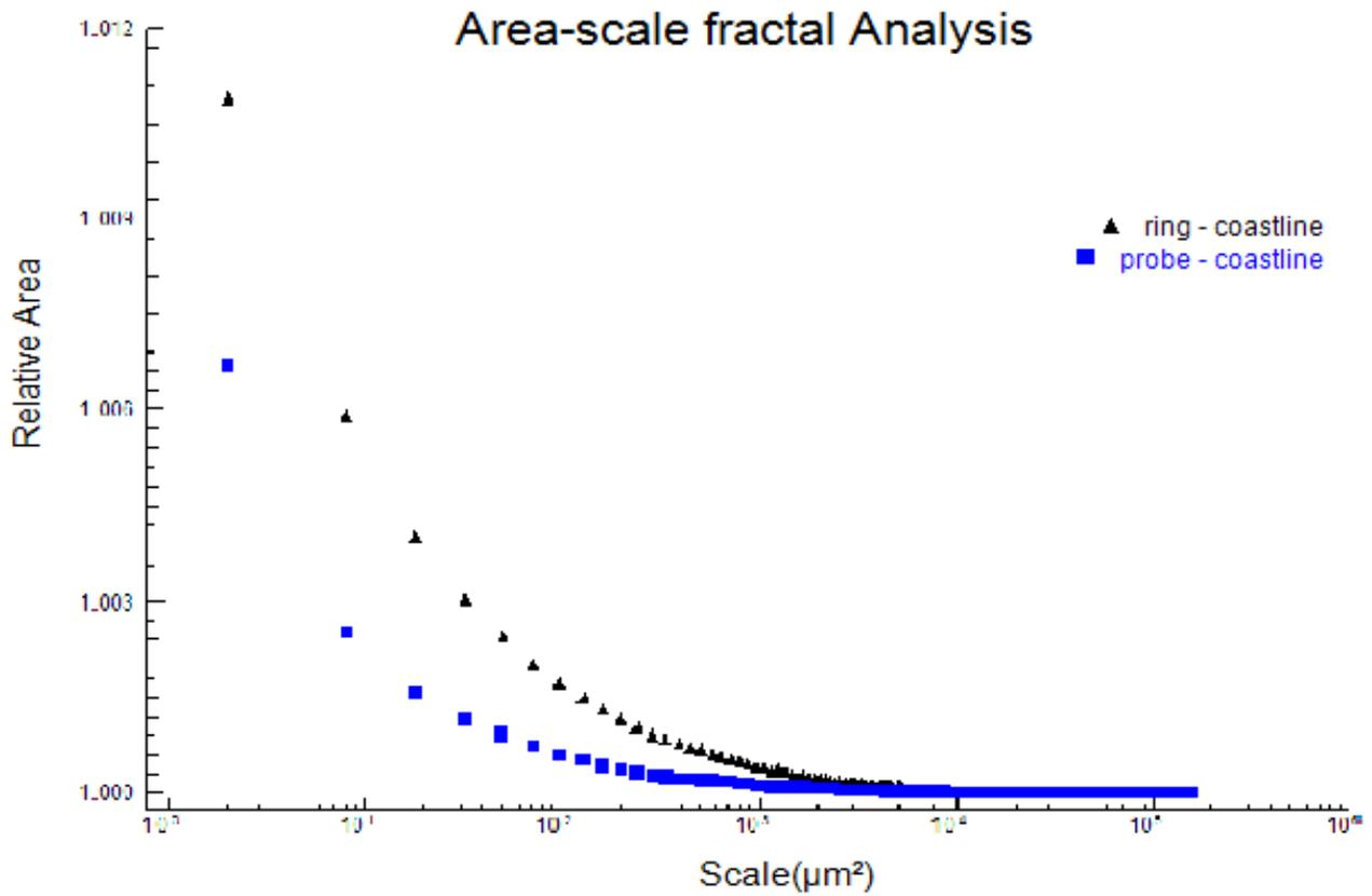
Figure 12. Surface roughness comparison for A 356 alloy.
