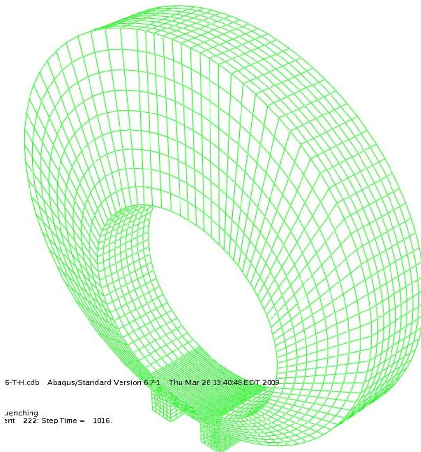
Figure 23. Refined mesh.
