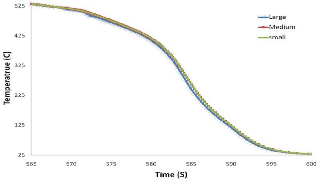
Figure 20. Cooling curves at the selected point obtained by simulation with different mesh densities.
