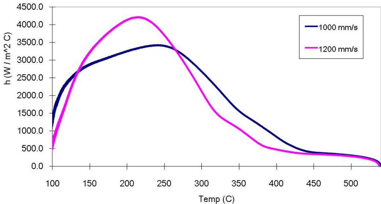
Figure 10. Calculated quenching heat transfer coefficient curves for A356 alloy.
