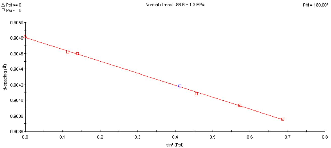
Figure 36. Change in d-spacing with  $\sin^2\psi$  for the horizontally quenched part.
