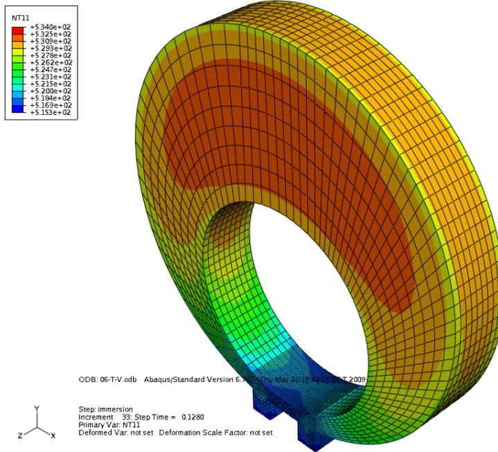
Figure 25. Thermal prediction for vertical quenching after immersion step.
