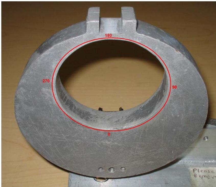
Figure 38. The path of CMM measurements.
