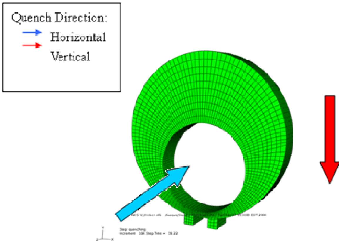
Figure 24. Schematic representation of the directions in which the parts were quenched.
