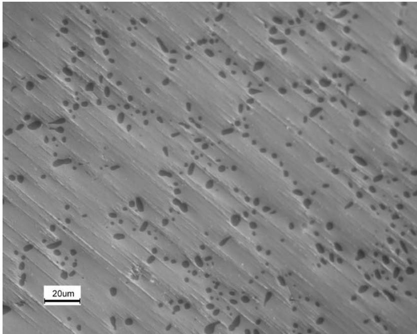
Figure 4. Microstructure of solutionized A356 alloy.
