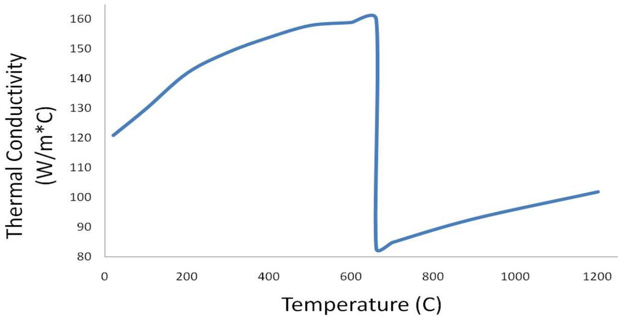
Figure 5. Calculated thermal conductivity as a function of temperature.
