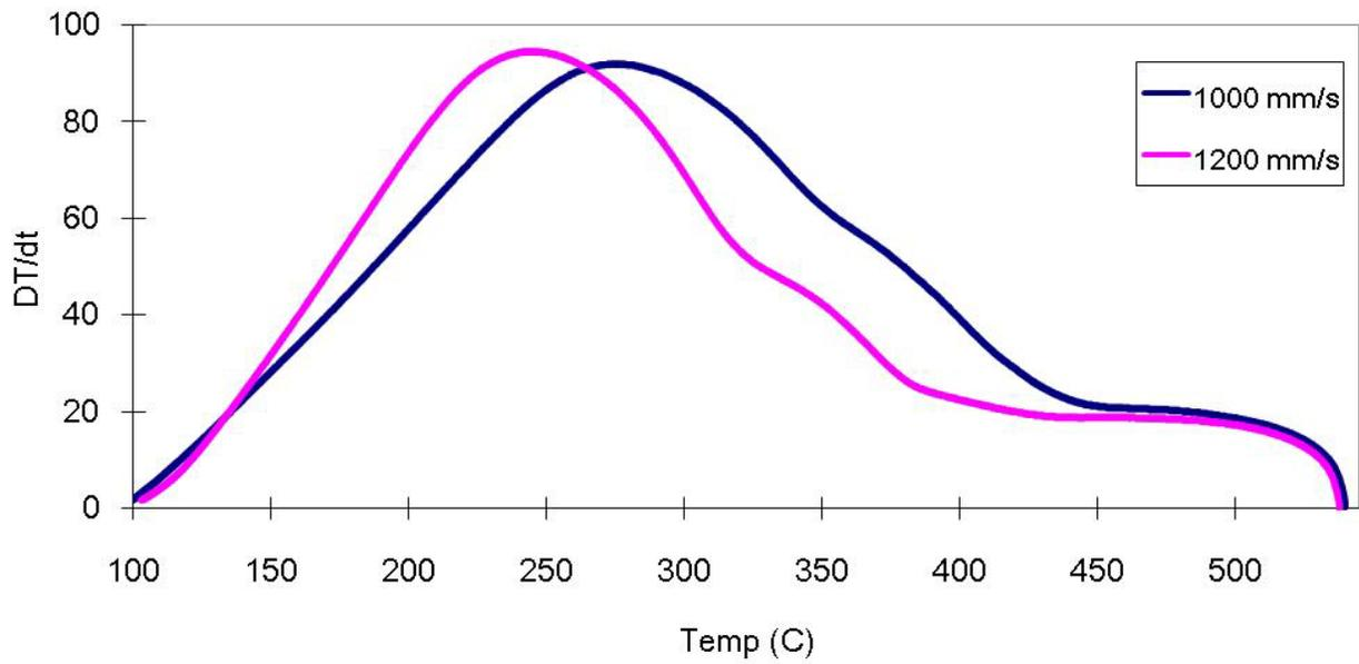
Figure 9. Calculated cooling rate vs. temperature for A356 alloy.
