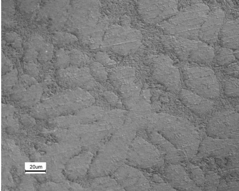
Figure 3. Microstructure of as-cast A356 alloy.
