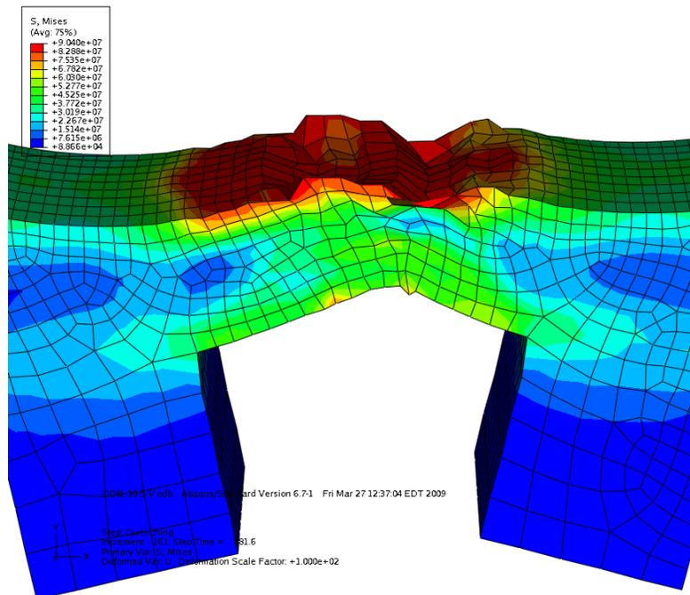
Figure 28. Thermal-stress prediction for vertical quenching after quenching step.
