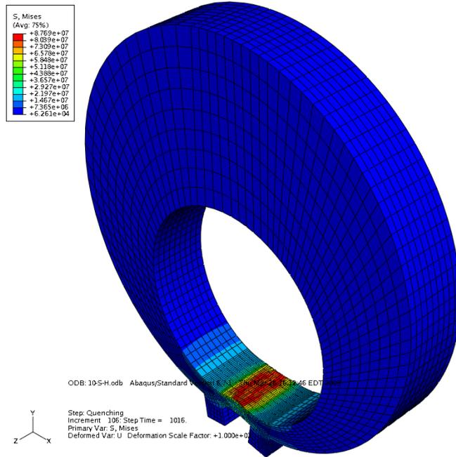
Figure 29. Thermal-stress prediction for horizontal quenching after quenching step.
