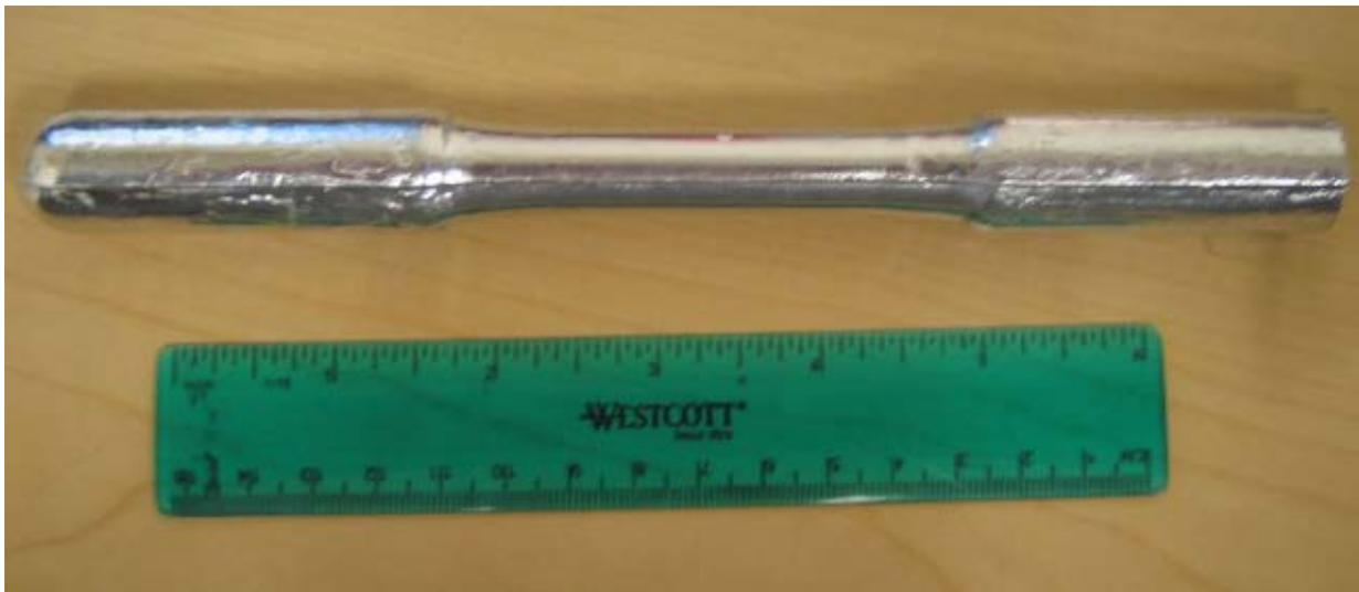
Figure 2. Cast A356.2 standard tensile bar.
