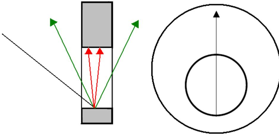
Figure 33. Diffractometer and location on the part where residual stresses were measured.
