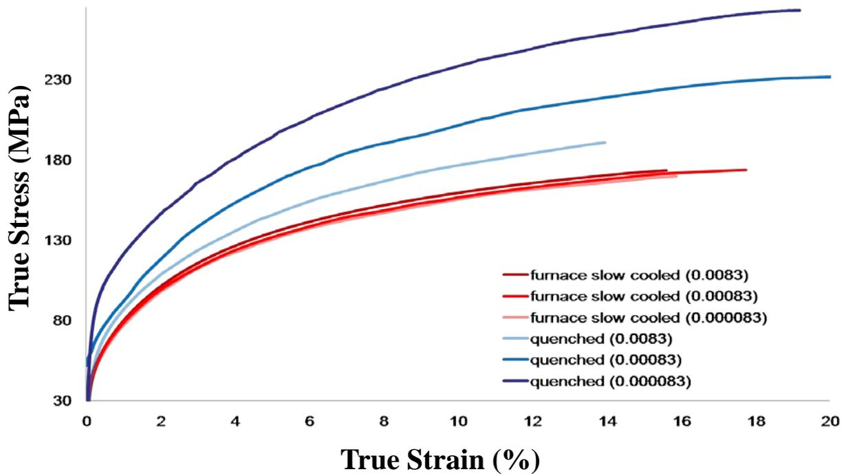
Figure 13. True stress-strain curves for water-quenched and slow-cooled samples at strain rates = 0.0083/s, 0.00083/s and 0.000083/s.
