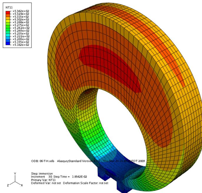
Figure 26. Thermal prediction for horizontal quenching after immersion step.
