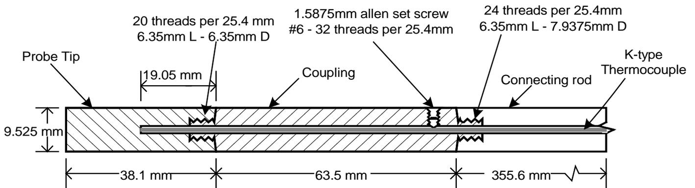
Figure 7. Quench probe-coupling-connecting rod assembly.
