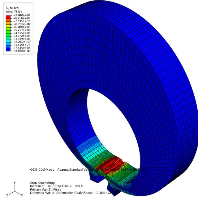
Figure 27. Thermal-stress prediction for vertical quenching after quenching step.
