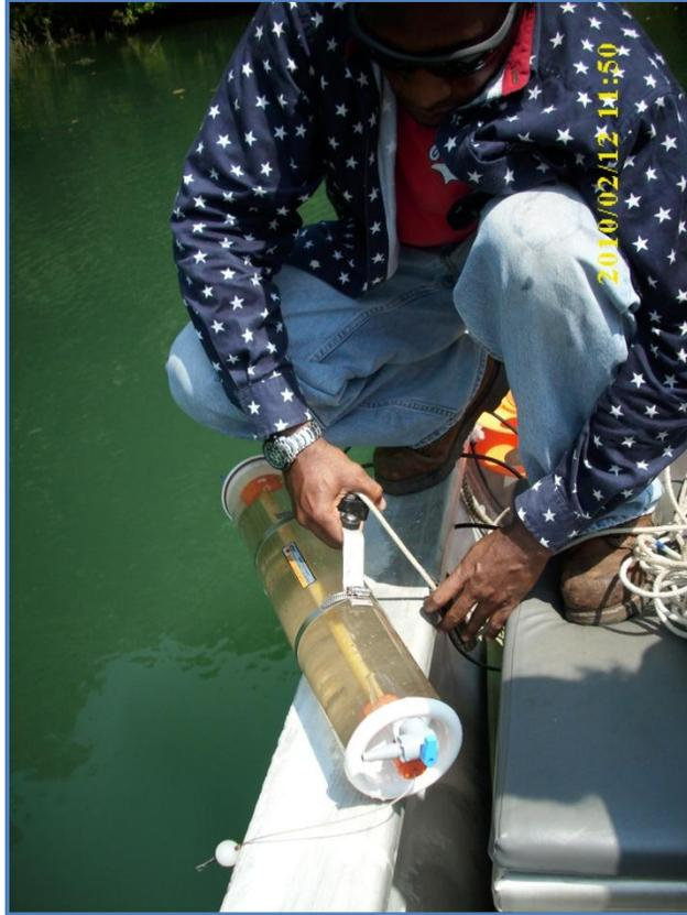
Figure D-7: Collection of Water Sample
