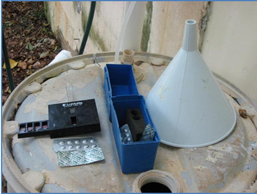
Figure A-9: Chlorine Testing Equipment
