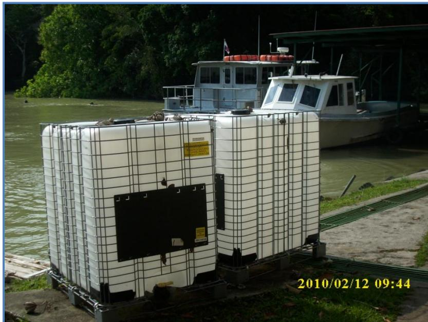
Figure C-2: 250 Gallon Tanks for Potable Water Storage for Transport, Feb. 12, 2010
