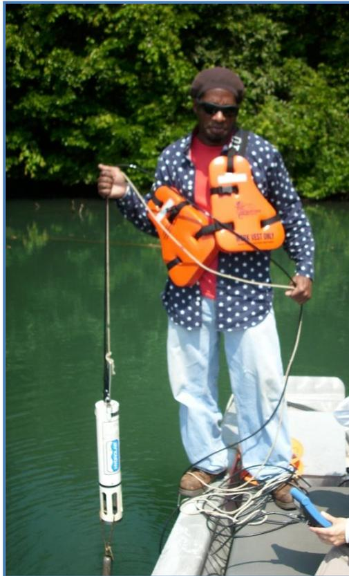
Figure D-4: Photo of Hydrolab DataSonde 4a Turbidimeter
