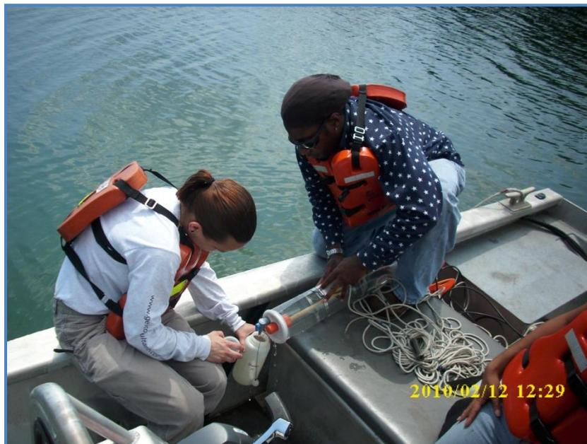
Figure D-8: Transferring Water from Van Dorn to Sample Container
