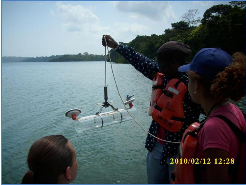
Figure D-5: Van Dorn Sediment Sampler
