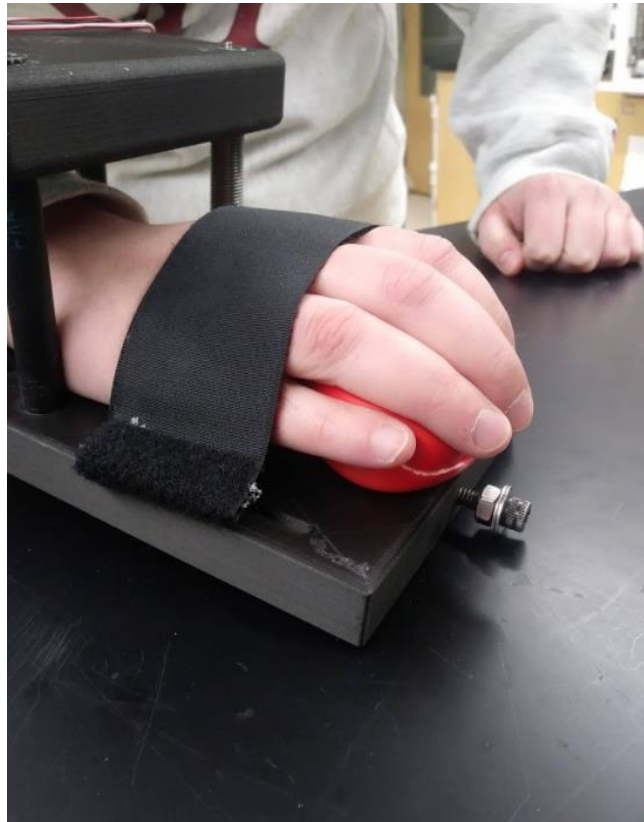
Figure 5 – Stress Ball Experimentation. This test was done to see how comfortable the patient’s hand was during testing, as well as the amount of restriction the patient had while holding the grip.
