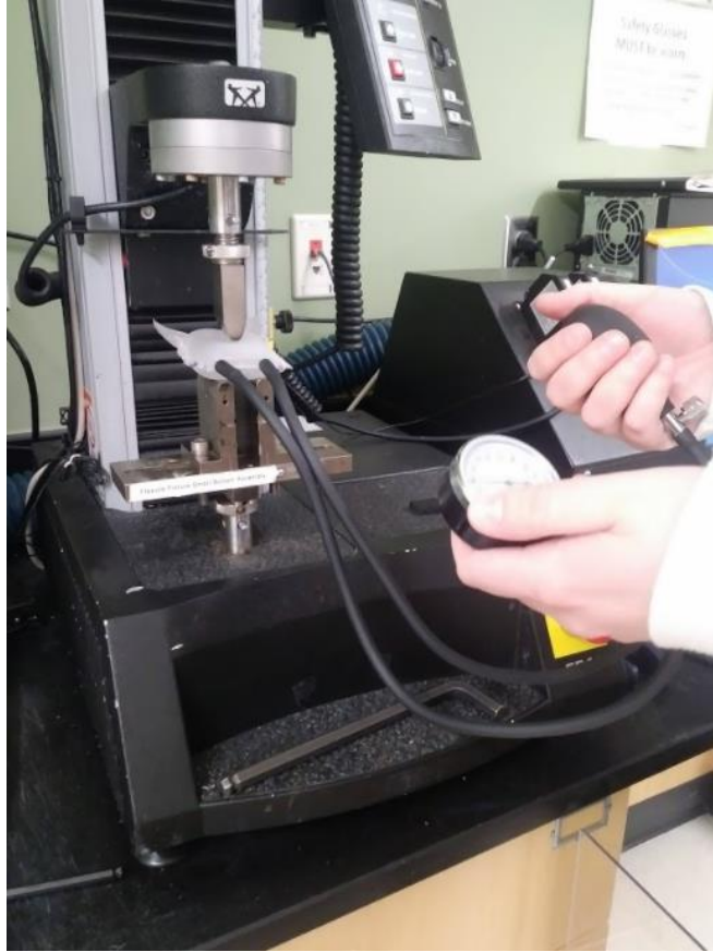
Figure 12 – Balloon Instron Testing. This test was done by pacing the balloon on the Instron and testing the force measured at each 20 mmHg interval.
