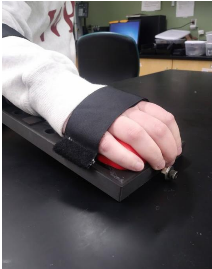
Figure 6 – Cut Stress Ball Experimentation. This test was done to see if the cut stress ball provided more comfort to the patient than the full stress ball.
