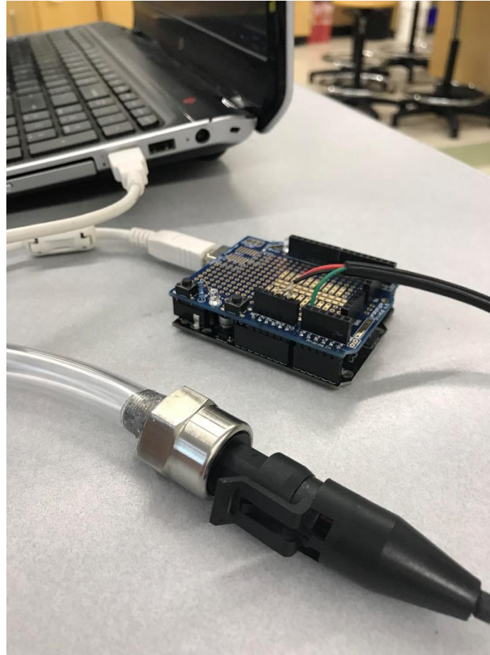
Figure 21 – Wired Arduino Assembly. This figure shows the pressure transducer which is connected to the Arduino which is then connected to a laptop. The Arduino was coded so that the data being transmitted to the laptop was instantaneous force application.
