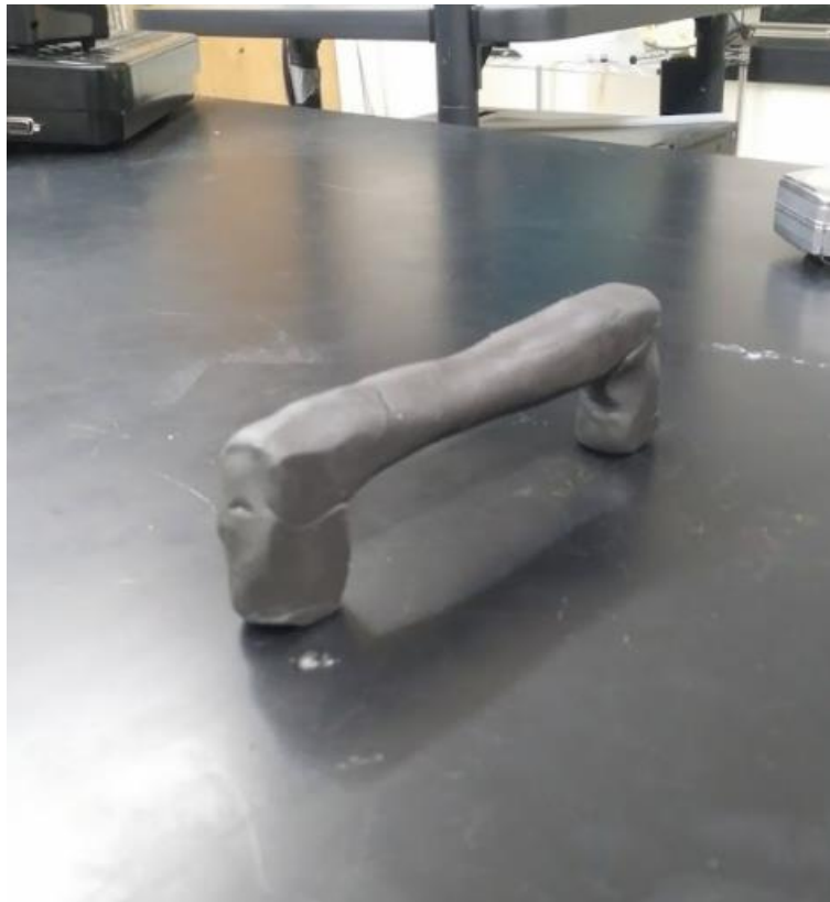
Figure 7 – Clay Modeled Grip. This grip was first modeled in clay to test the comfort of the grip before 3D printing.
