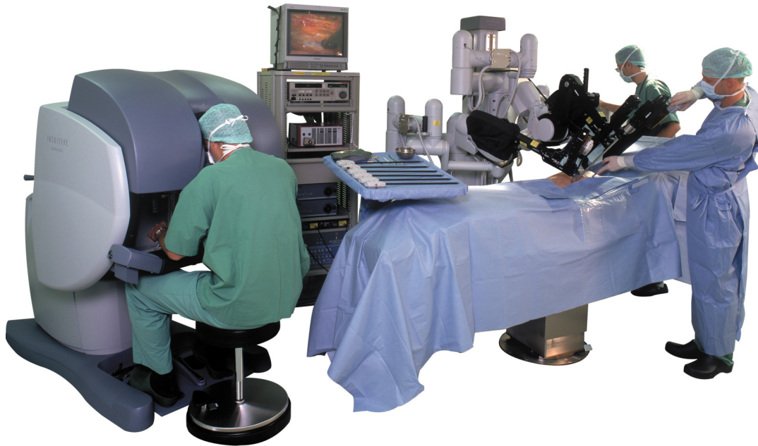
Figure 1.6: The da Vinci Surgical System with the surgeon operating the MTM console and the helping nurse at the PSM station
