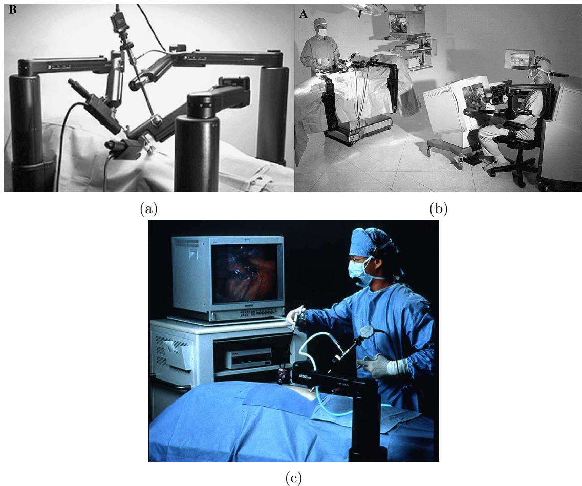
Figure 1.5: (a) The ZEUS Slave Console.(b) The ZEUS system with Master and Slave Console.(c) The automated endoscope called (AESOP)
