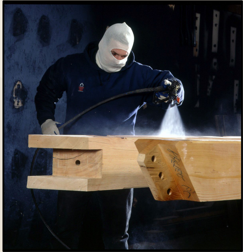
Application Process of Wood Sealer
