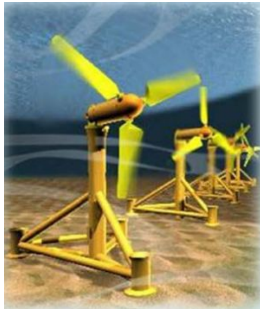
[34] Image Courtesy of U.S. Department of Energy: Model of an underwater ocean current energy turbine.
