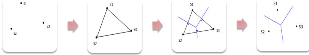
Figure 2.3: Voronoi Triangulation creation from a set of points
