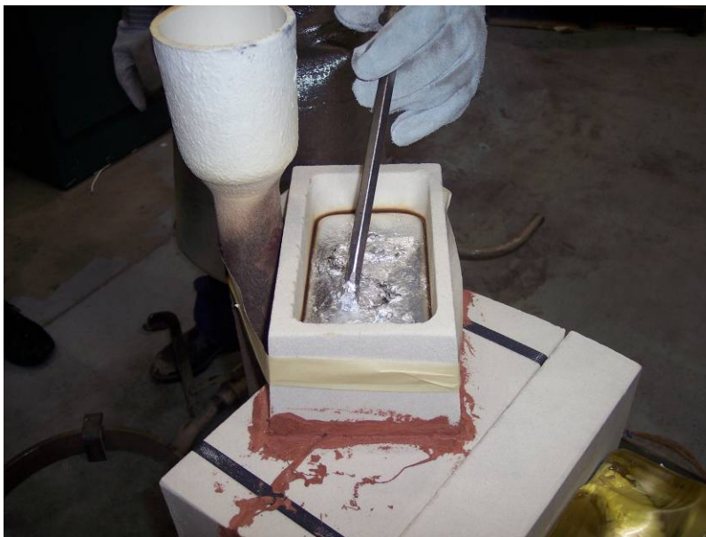
MCT foundry worker demonstrating the “stickiness” of molten aluminum
