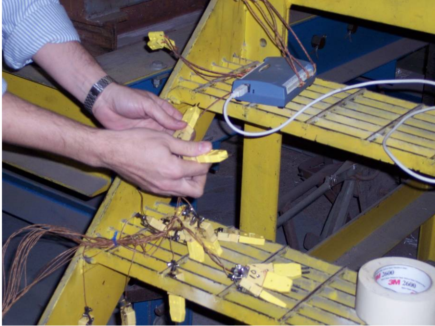
Scott's hands trying to make the thermocouple system work correctly
