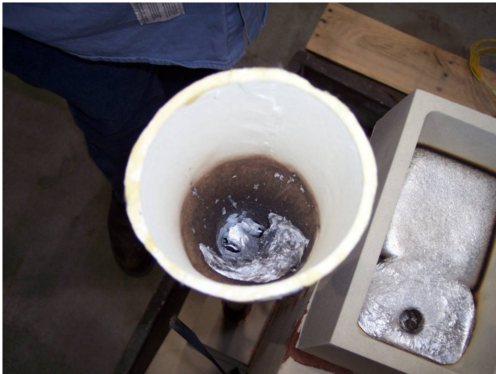
View of down-sprue after aluminum has been poured
