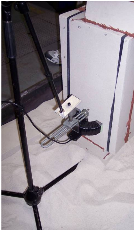
Figure 3.13: Single coil support structure placed by sand mold
