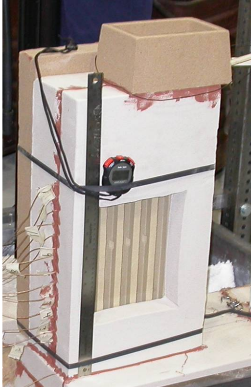
Close-up view of glass window on the sand mold
