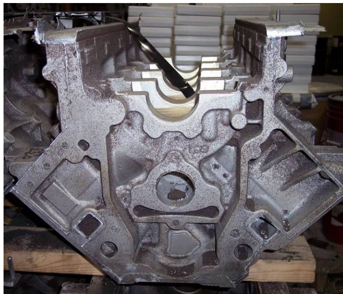
Figure 1.1: Side profile of a V-block engine (upside-down)
