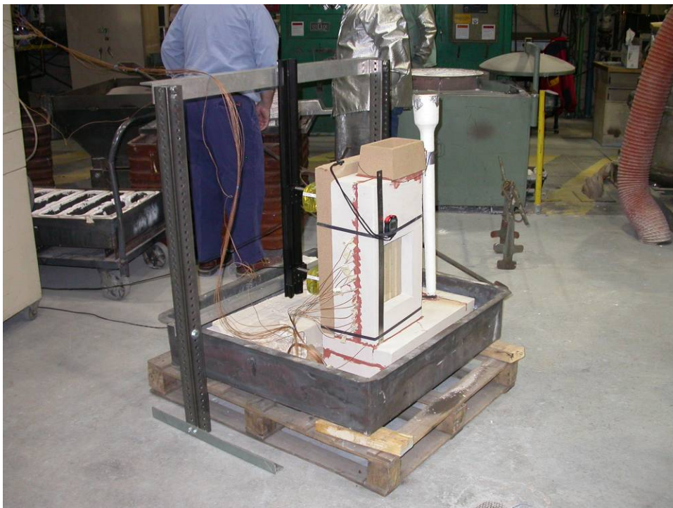
View of sand mold with glass window to view the molten aluminum
