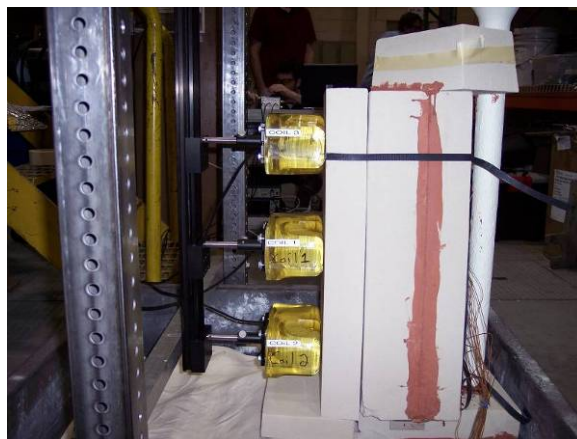
Figure 3.21: Coil support structure in use for a test
