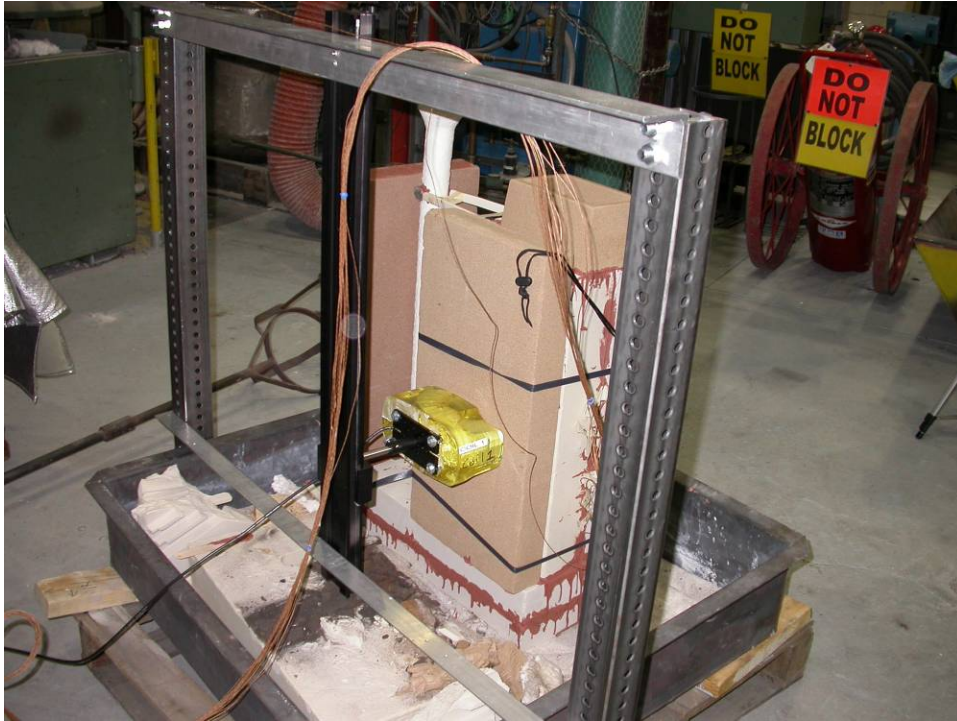
View of sand mold set up and ready to be poured
