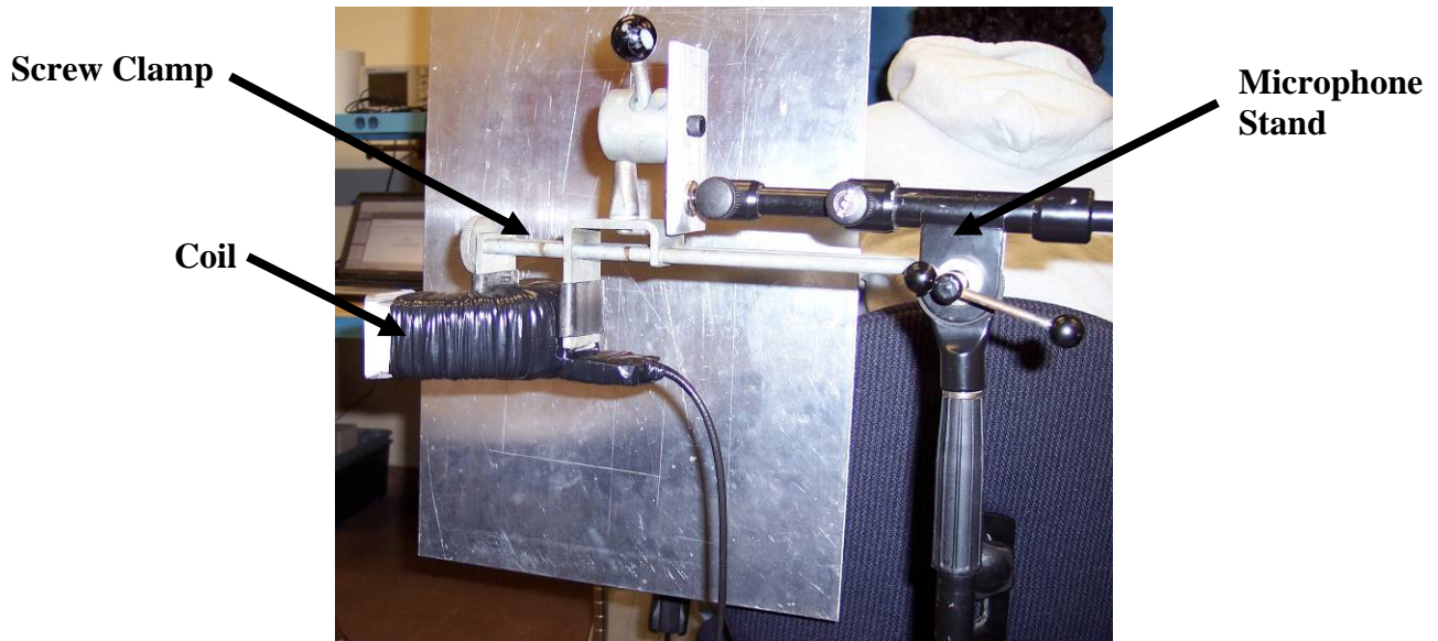
Figure 3.12: Single coil support structure close-up
