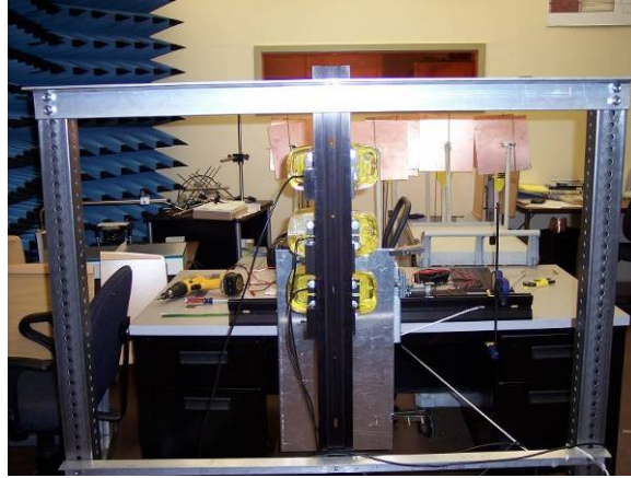
Figure 3.20: Completed tri-coil support structure - rear view
