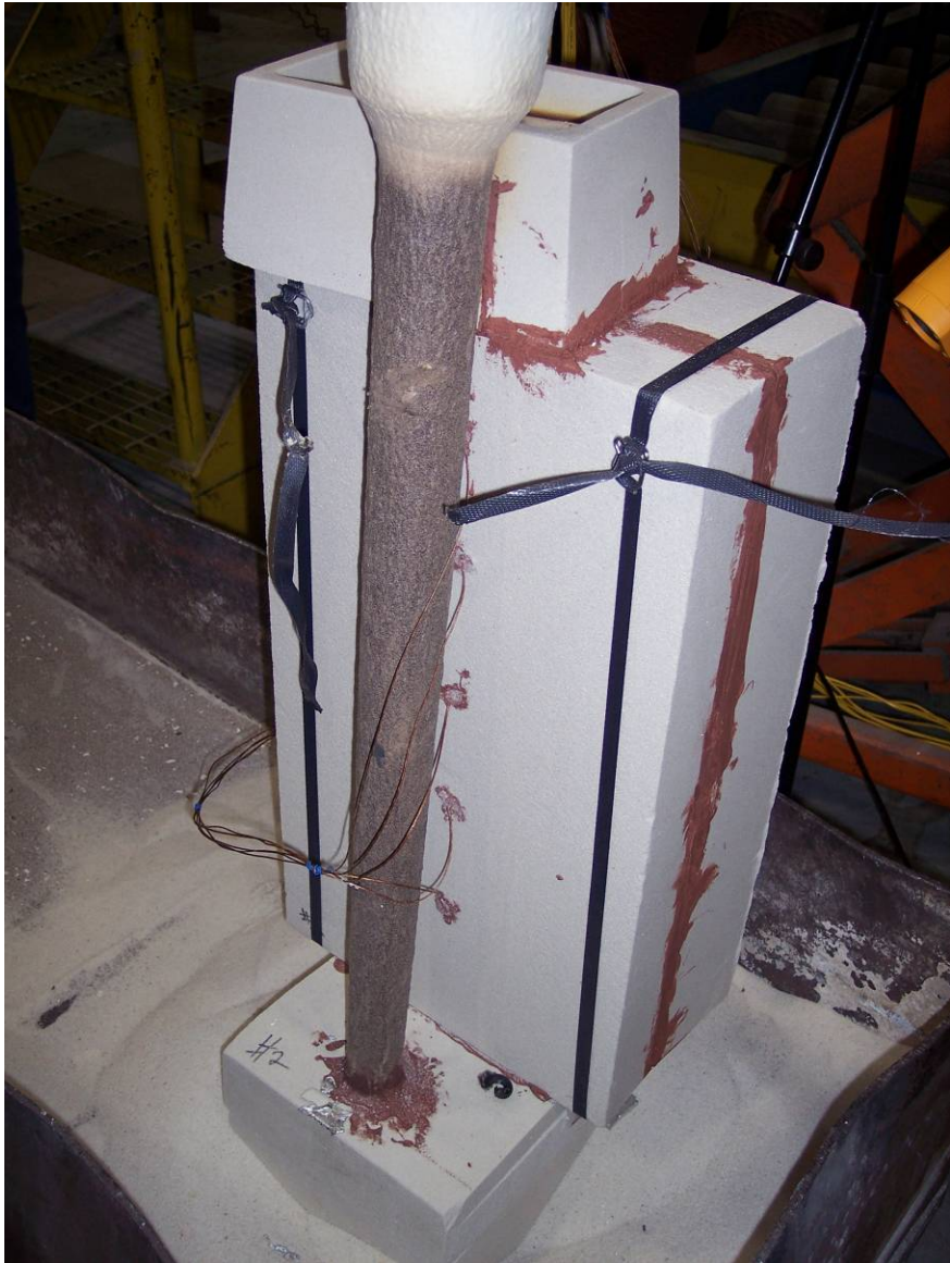
Mold after being filled with molten aluminum
