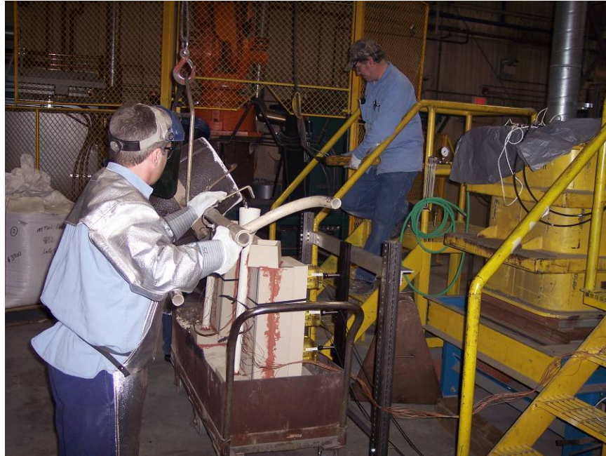
Foundry workers pouring molten aluminum into sand cast used for testing
