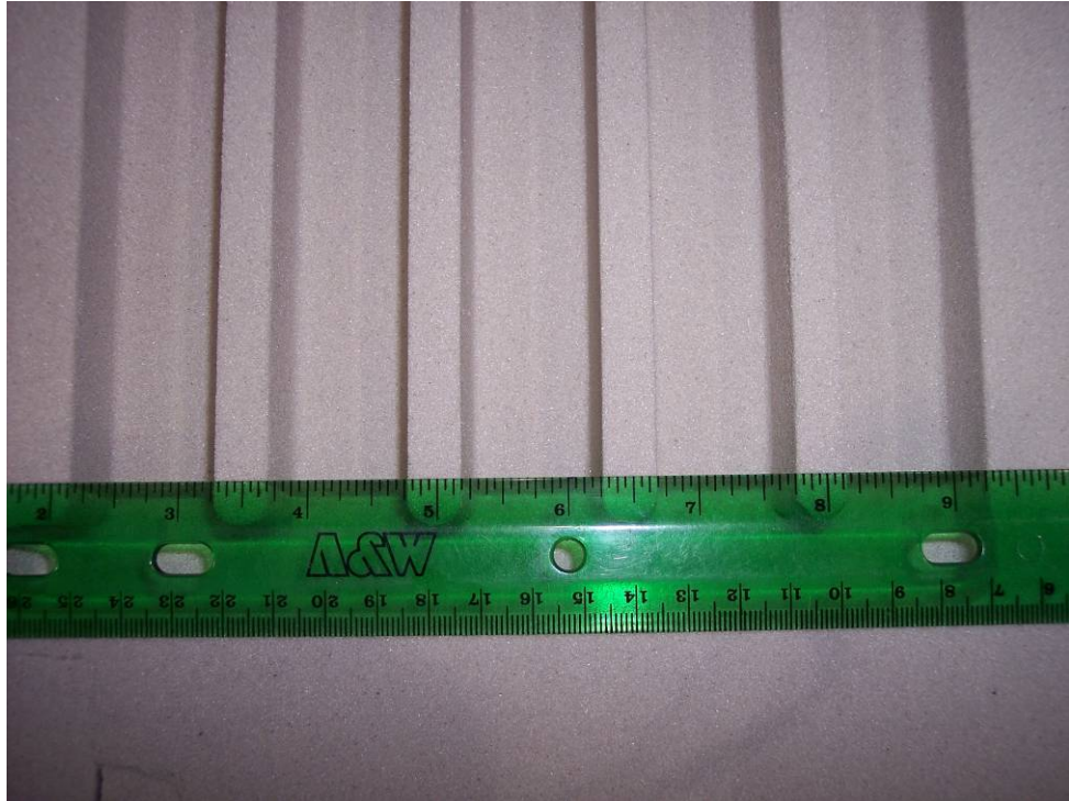
Inside details of sand mold close-up
