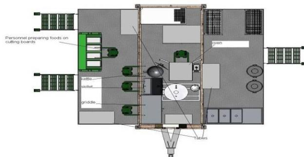
**Figure 4.3.1 Lay-out of Containerized Kitchen**
