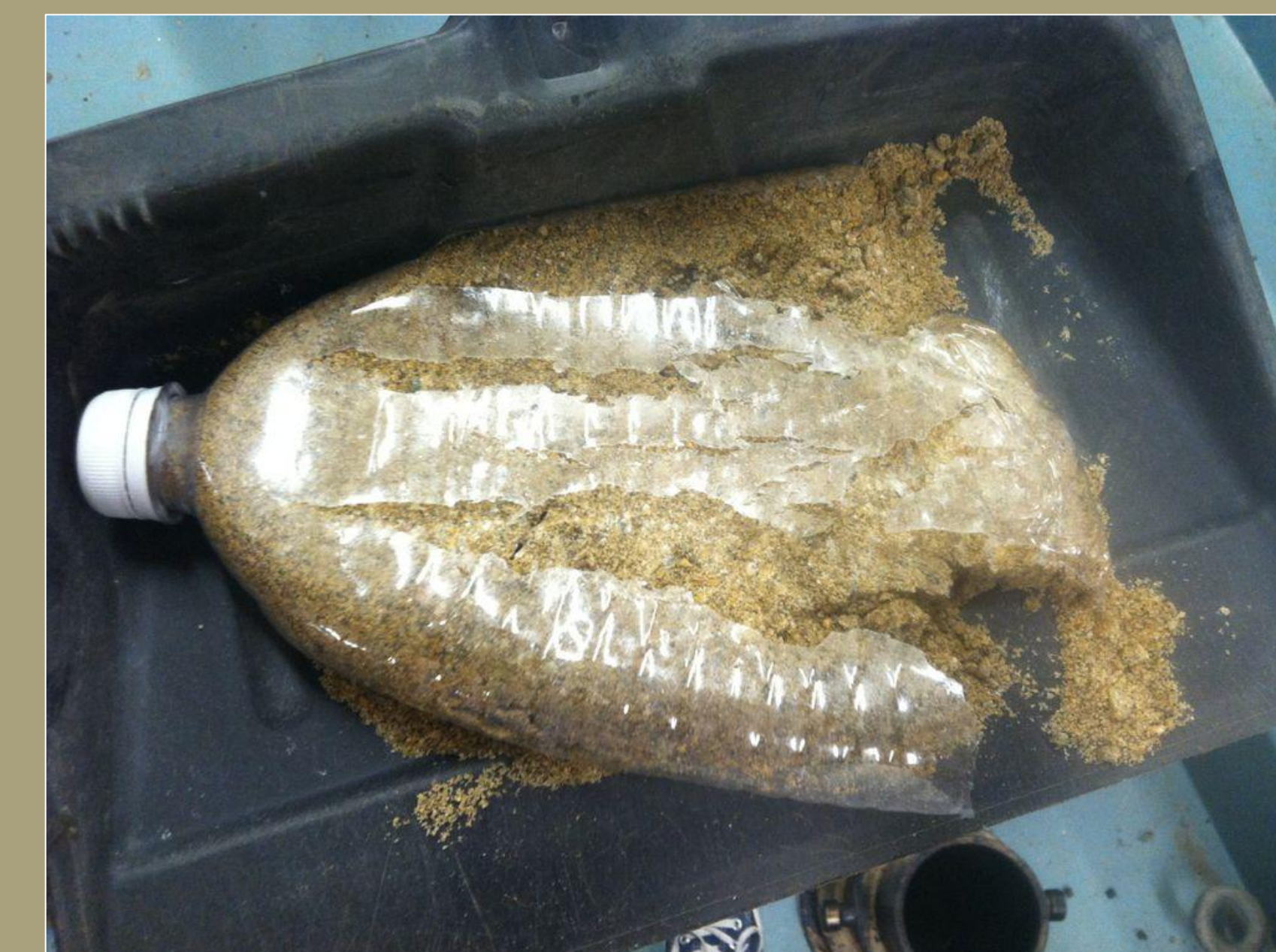
A half liter bottle filled with sand after the compression test
