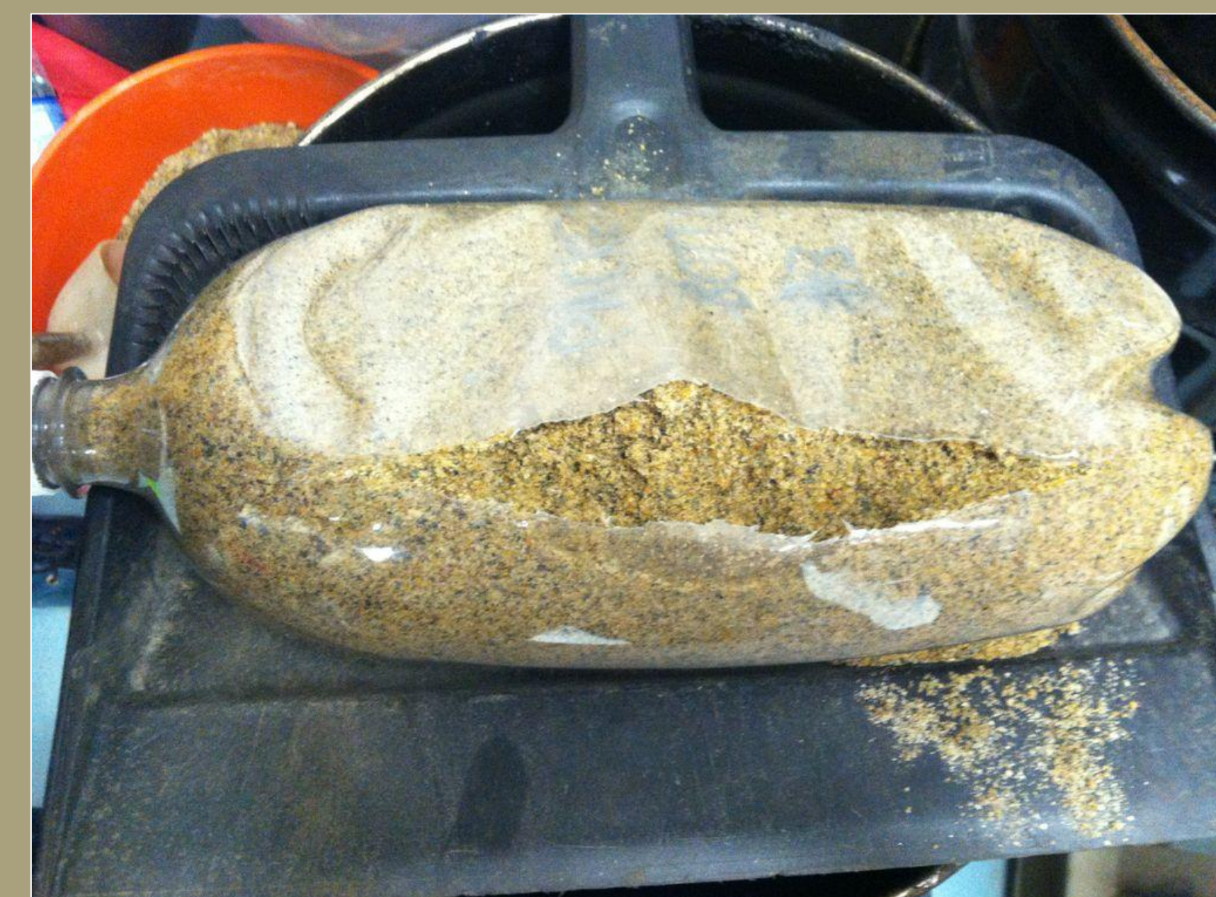
A 2 liter bottle tightly packed with sand after the compression test
