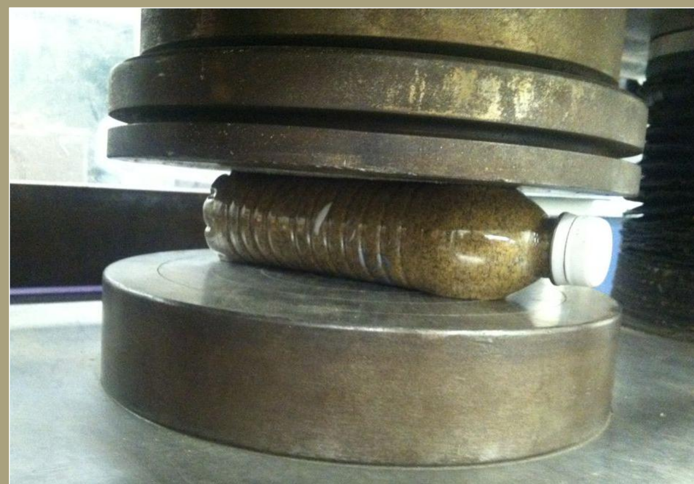
A compression test on a half liter bottle tightly packed with sand.
