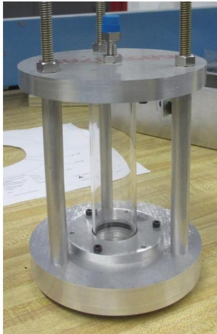
**Figure 19.** Completed thruster mechanical assembly.
