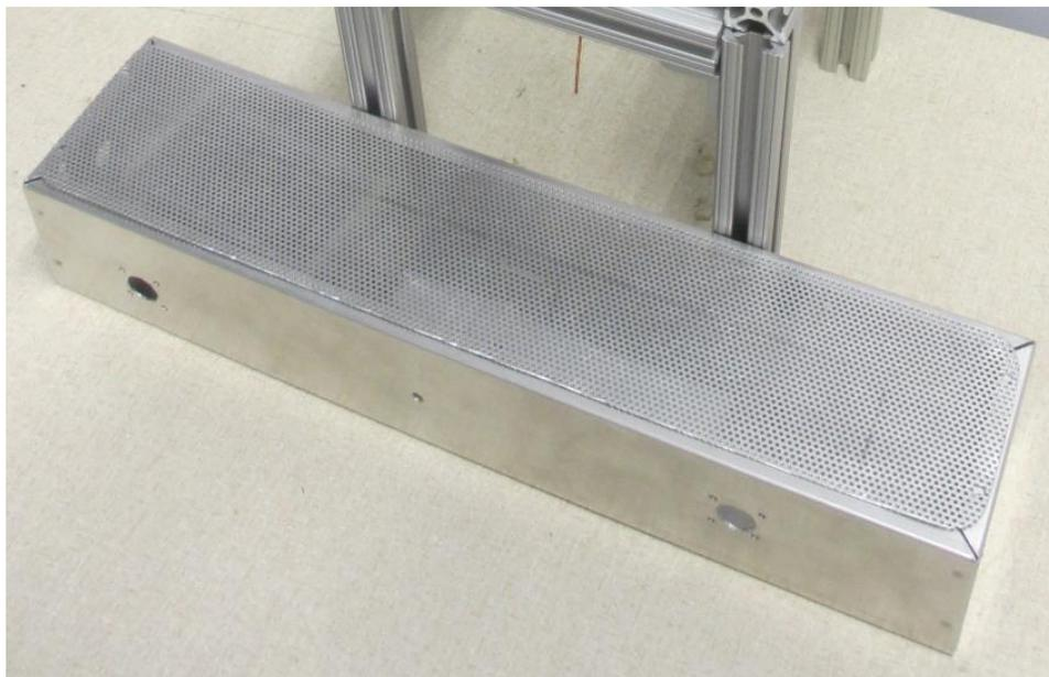
**Figure 26.** Matching network enclosure assembly, without lid fasteners in place.
