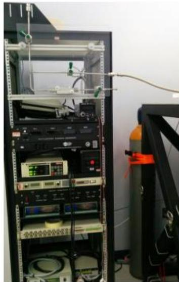
**Figure 31.** Instrument Panel Showing Flow Control Panel and Argon Tank In Final Location [1].
