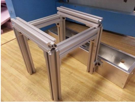
**Figure 40.** Assembled Stand Attached to Matching Network Enclosure
