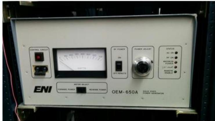
**Figure 30.** ENI OEM-650A RF Power Supply [1].
