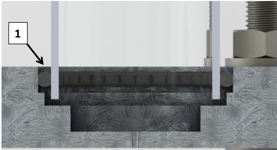
**Figure 12.** Cross-section of discharge chamber tube, end-plate seal from 2015 RFET MQP [1].
