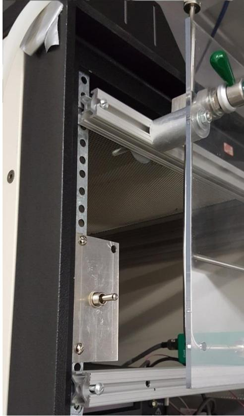
**Figure 41.** Switch mounted to Control Panel.
