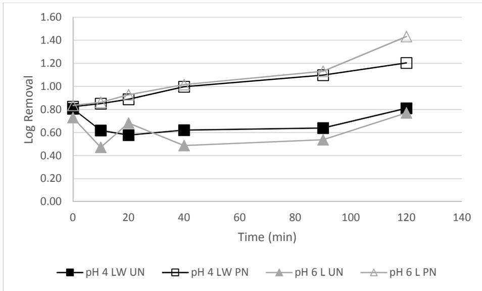
Figure 7-3: Average Log Removals of particles with sand in lab water with (1) pH 4 and (2) pH 6
