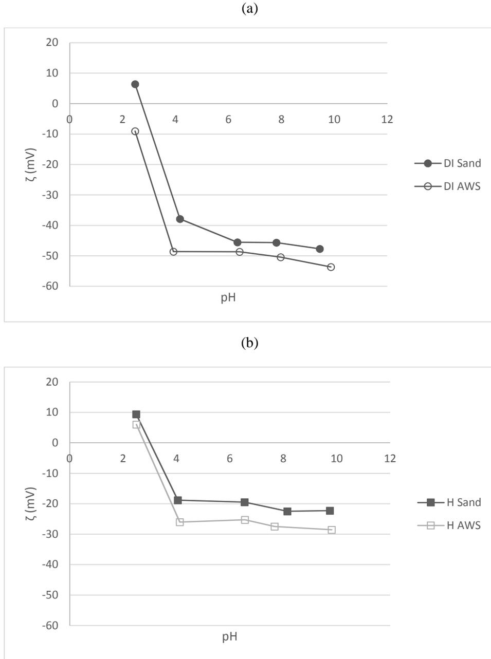
Figure 7-5: Zeta Potentials of Sand and Acid-Washed Sand in (a) Lab Water and (b) High Ionic Strength Solution
