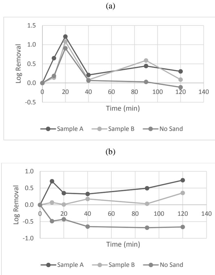
Figure 6-5: Log Removals of MS2 with Sand Media in Low Ionic Strength Water at (a) pH 6 and (b) pH 8
