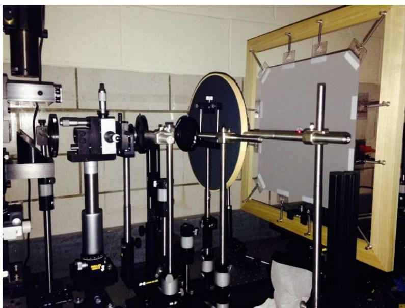
Figure 5-8: ARGOS Set-Up Portraying the Laser, Lens, Filters, Sample Holder and Front of Screen
