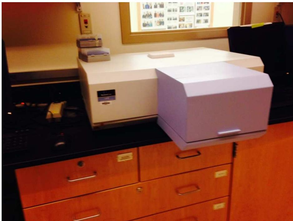
Figure 5-5: Fluorescence Spectrophotometer
