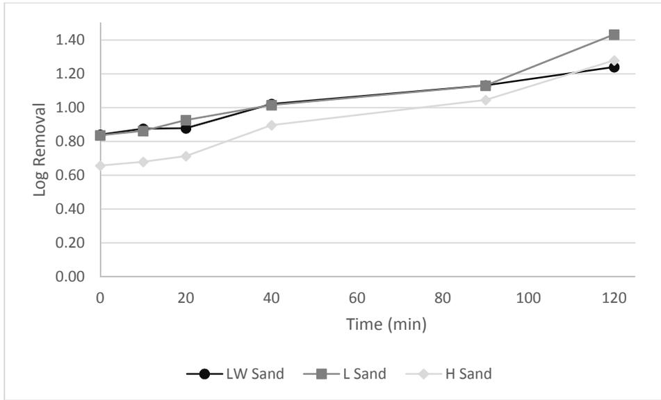
Figure 7-2b: Average Log Removals with Sand and Varied Ionic Strength for Protein-Coated Nanoparticles
