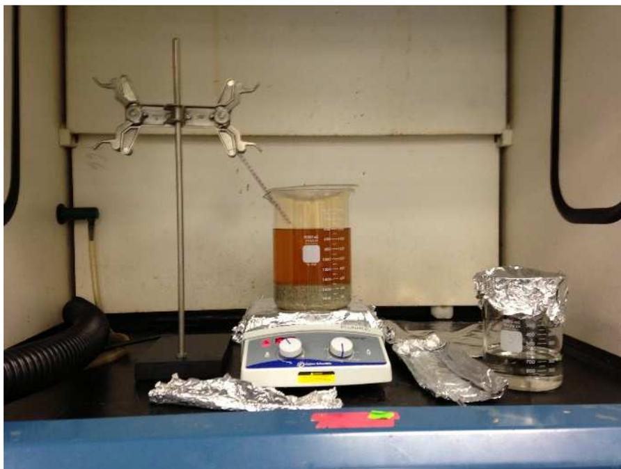
Figure 5-6: Sand Media Prepared in Concentrated Acid
