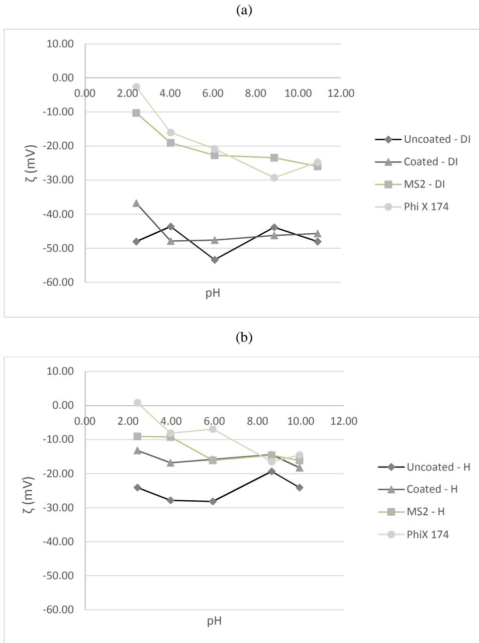
Figure 7-6: Average Zeta Potentials of Particles in Solutions for 2.5 to 10 in (a) Lab Water and (b) High Ionic Strength Water
