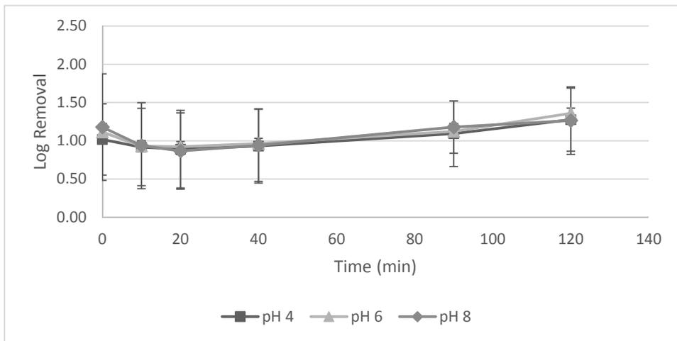
Figure 6-1: Log Removals in pH 4, 6, 8 for Uncoated Particles with Sand Media (a) Lab water (b) Low Ionic Strength Water (c) High Ionic Strength Water (error bars represent standard deviation, n=8)
