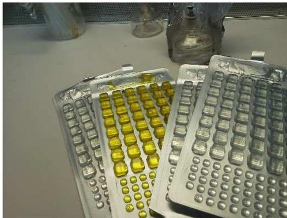
Figure 5-3: Coliform Enumeration Quantitrays
