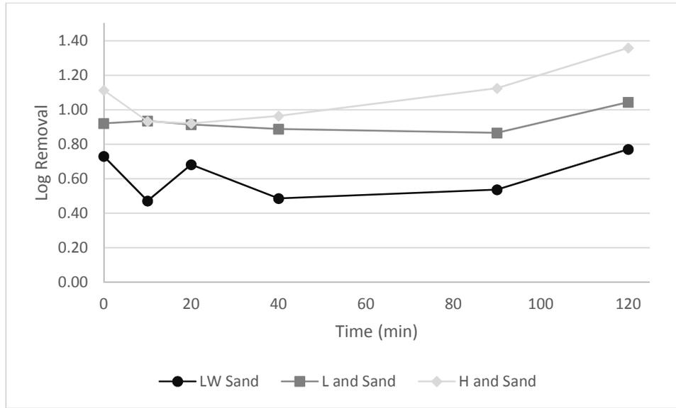
Figure 7-2a: Average Log Removals with Sand and Varied Ionic Strength for Uncoated Nanoparticles
