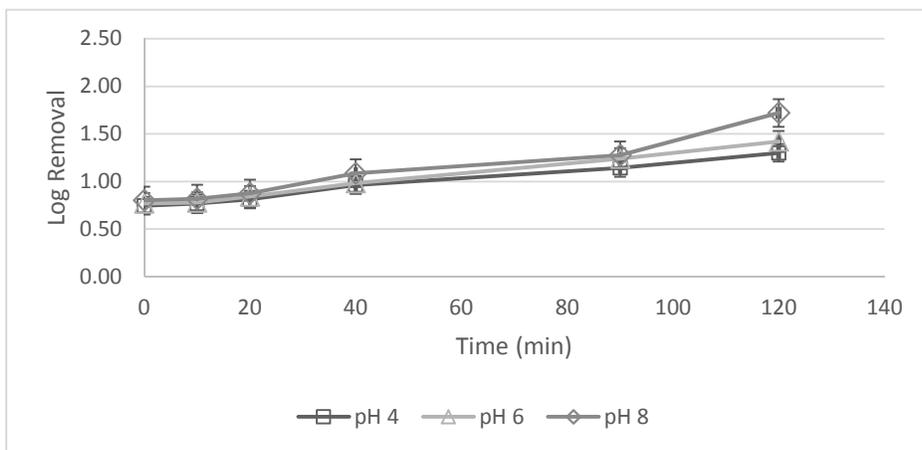
Figure 6-4: Log Removals in pH 4, 6, 8 for Protein Coated Nanoparticles with Sand Media (a) Lab Water (b) Low Ionic Strength Water (c) High Ionic Strength Water (error bars represent standard deviation, n=8)
