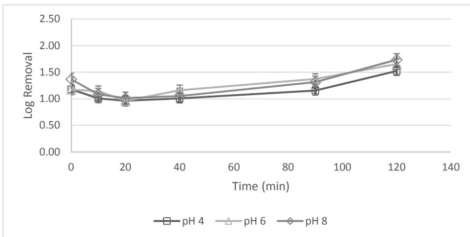
Figure 6-2: Log Removals in pH 4, 6, 8 for Uncoated Particles with Acid Washed Sand Media (a) Lab Water (b) Low Ionic Strength Water (c) High Ionic Strength Water (error bars represent standard deviation, n=8)
